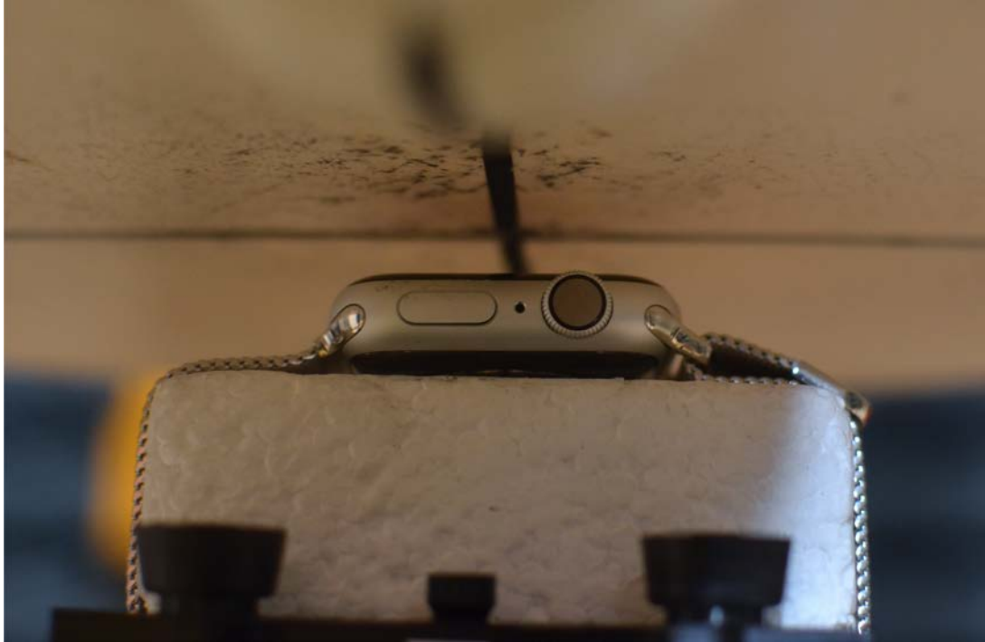
SAR Test Setup Photo 3: Aluminum front side at 1.0 cm with metal Loop wrist band
