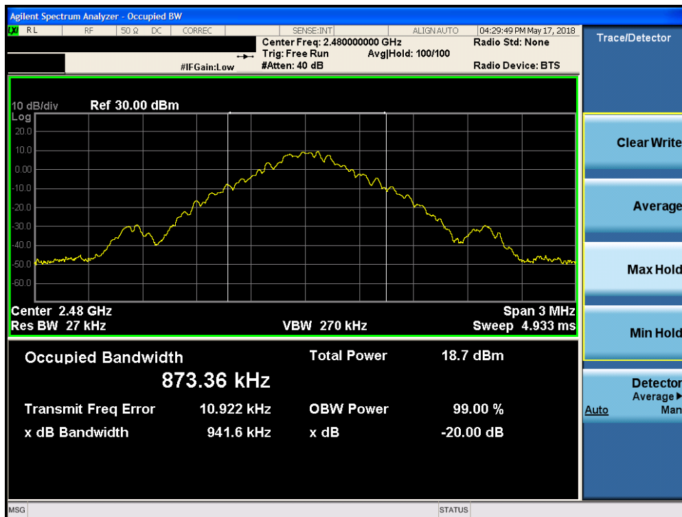
Plot 7-6. 20dB Bandwidth Plot (Bluetooth, GFSK, iPA – Ch. 78)
