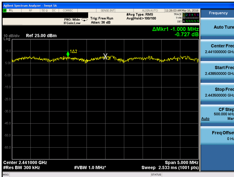
Plot 7-42. Channel Spacing Plot (Bluetooth, 8DPSK, ePA)
