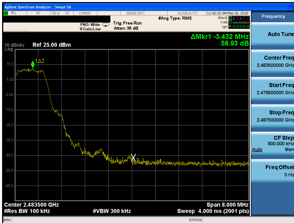
Plot 7-34. Band Edge Plot (Bluetooth with Hopping Disabled, 8DPSK, ePA – Ch. 78)
