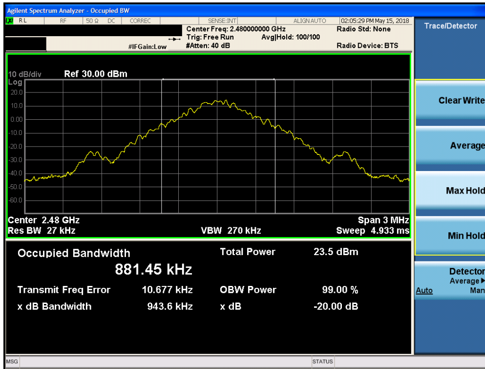
Plot 7-3. 20dB Bandwidth Plot (Bluetooth, GFSK, ePA – Ch. 78)
