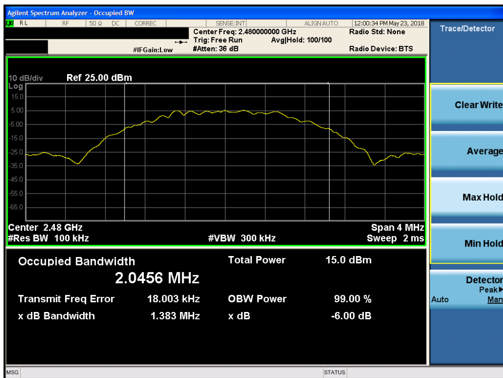
Plot 7-12. 6dB Bandwidth Plot (Bluetooth (LE), 2Mbps, iPA – Ch. 39)
