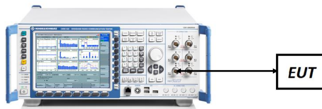
Figure 7-4. Conducted Power Measurement Setup
