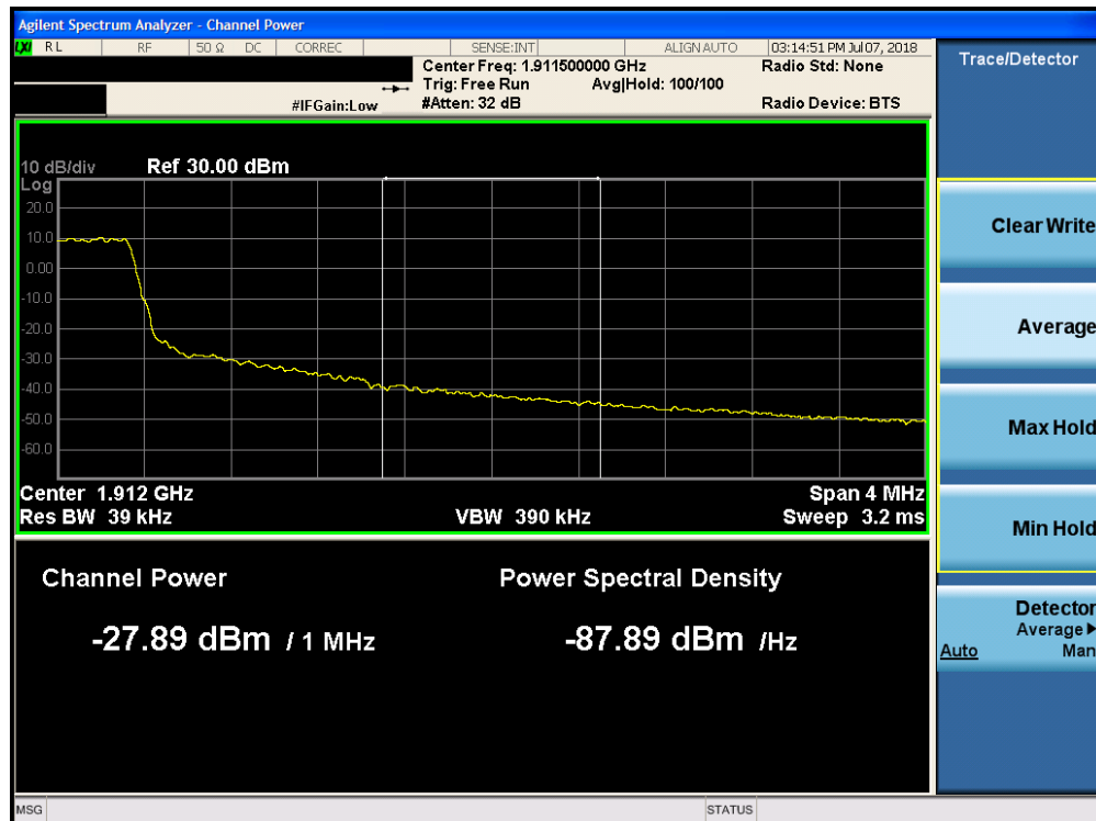
Plot 7-249. Upper Extended Band Edge Plot (Band 2 - 1.4MHz QPSK - Full RB Configuration)
