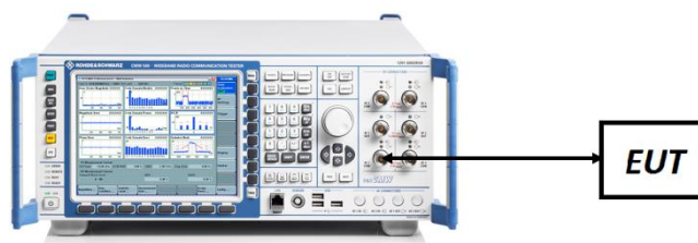
Figure 7-5. ERP/EIRP Measurement Setup
