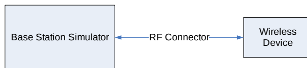
Figure 8-1 Power Measurement Setup
