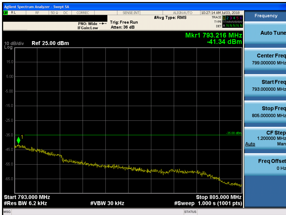
Plot 7-177. Upper Emission Mask Edge Plot (Band 13 - 10.0MHz QPSK - Full RB Configuration)
