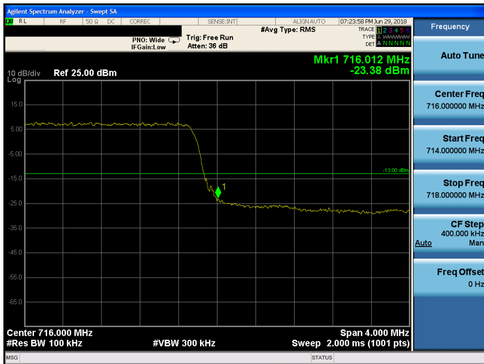
Plot 7-167. Upper Band Edge Plot (Band 17 - 5.0MHz QPSK - Full RB Configuration)
