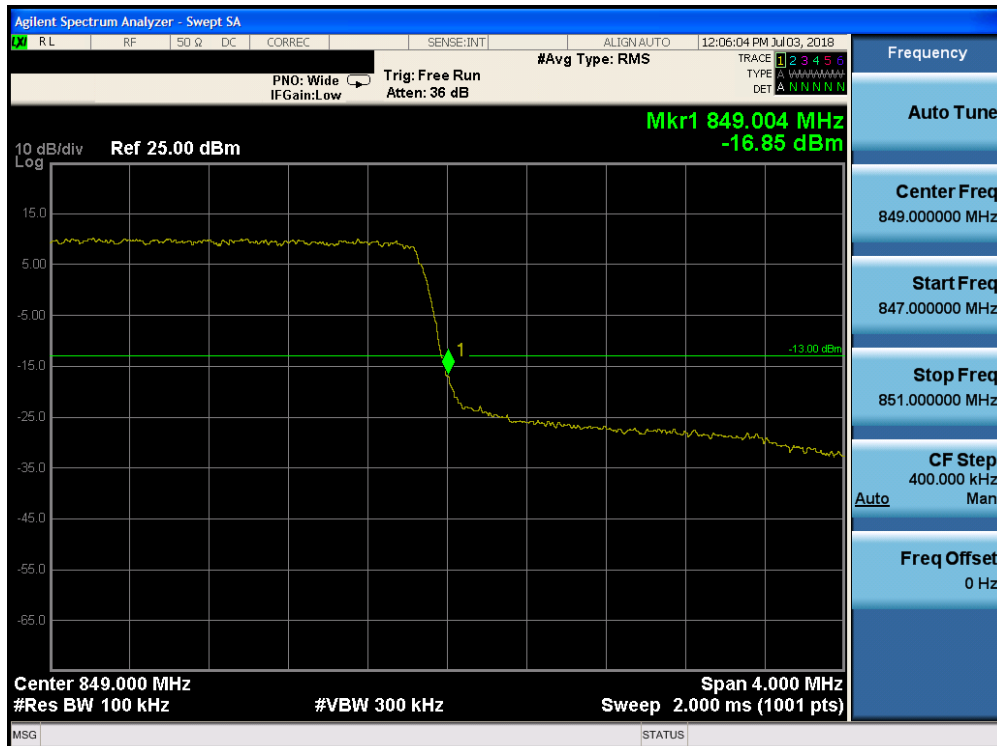
Plot 7-189. Upper Band Edge Plot (Band 5 - 3.0MHz QPSK - Full RB Configuration)
