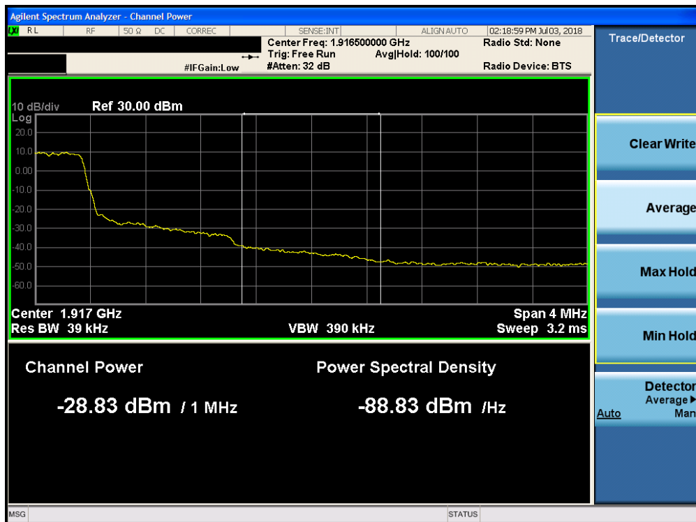
Plot 7-221. Upper Extended Band Edge Plot (Band 25 - 1.4MHz QPSK - Full RB Configuration)
