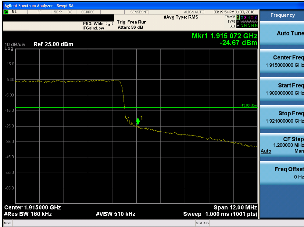
Plot 7-236. Upper Band Edge Plot (Band 25 - 15.0MHz QPSK - Full RB Configuration)
