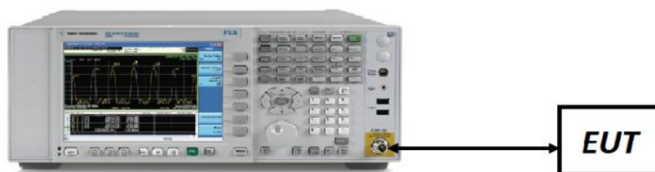
Figure 7-4. Test Instrument & Measurement Setup
