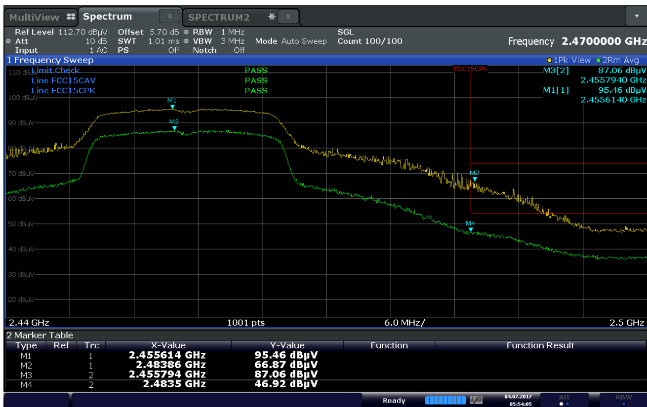
Plot 7-46. Radiated Restricted Upper Band Edge Measurement (Average & Peak)
