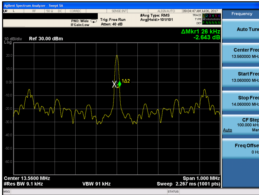
Figure 7-4. 20dB Bandwidth Plot (CE F 424kbps)
