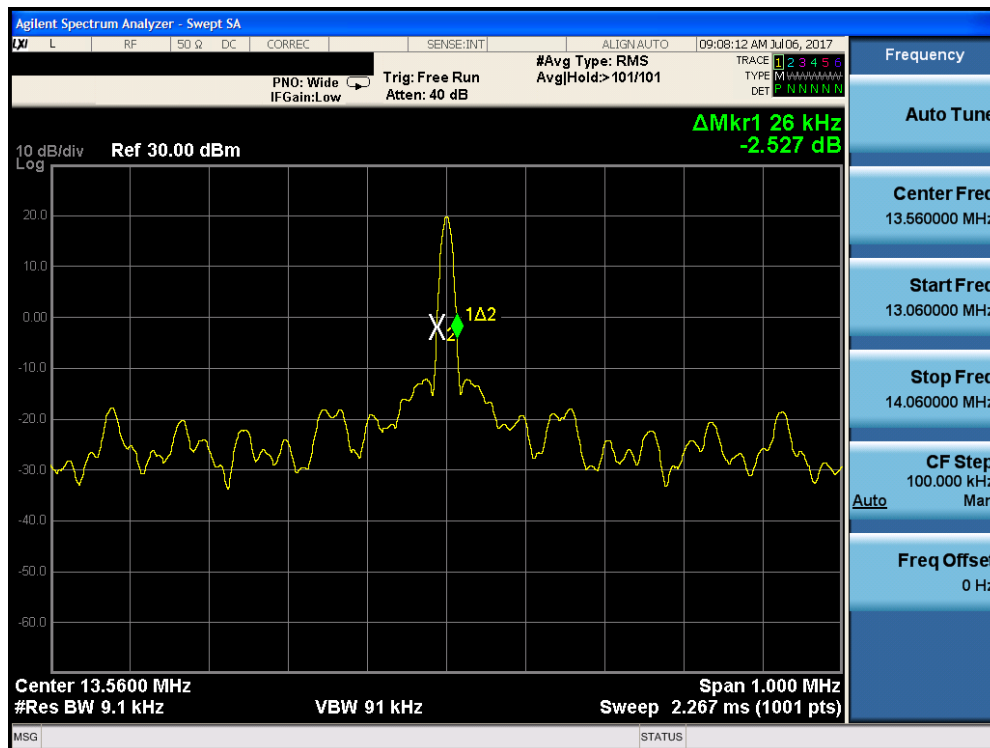
Figure 7-3. 20dB Bandwidth Plot (CE B 848kbps)
