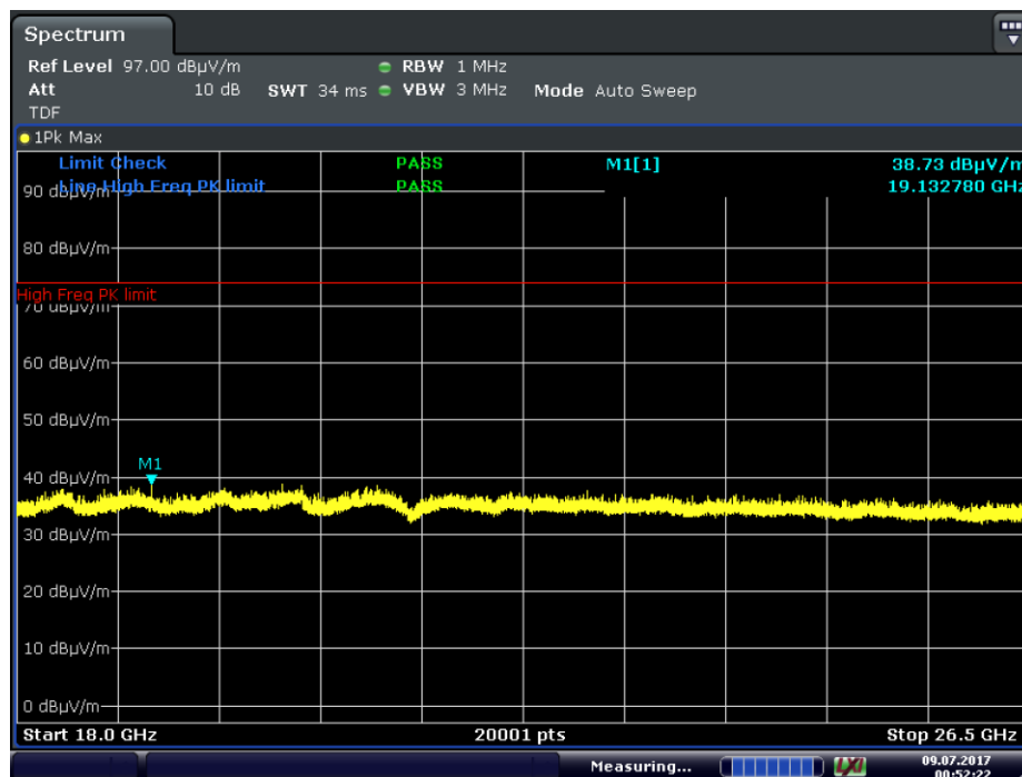
Plot 7-40. Radiated Spurious Plot above 18GHz (802.11b – Ch. 6, Ant. Pol. H)
