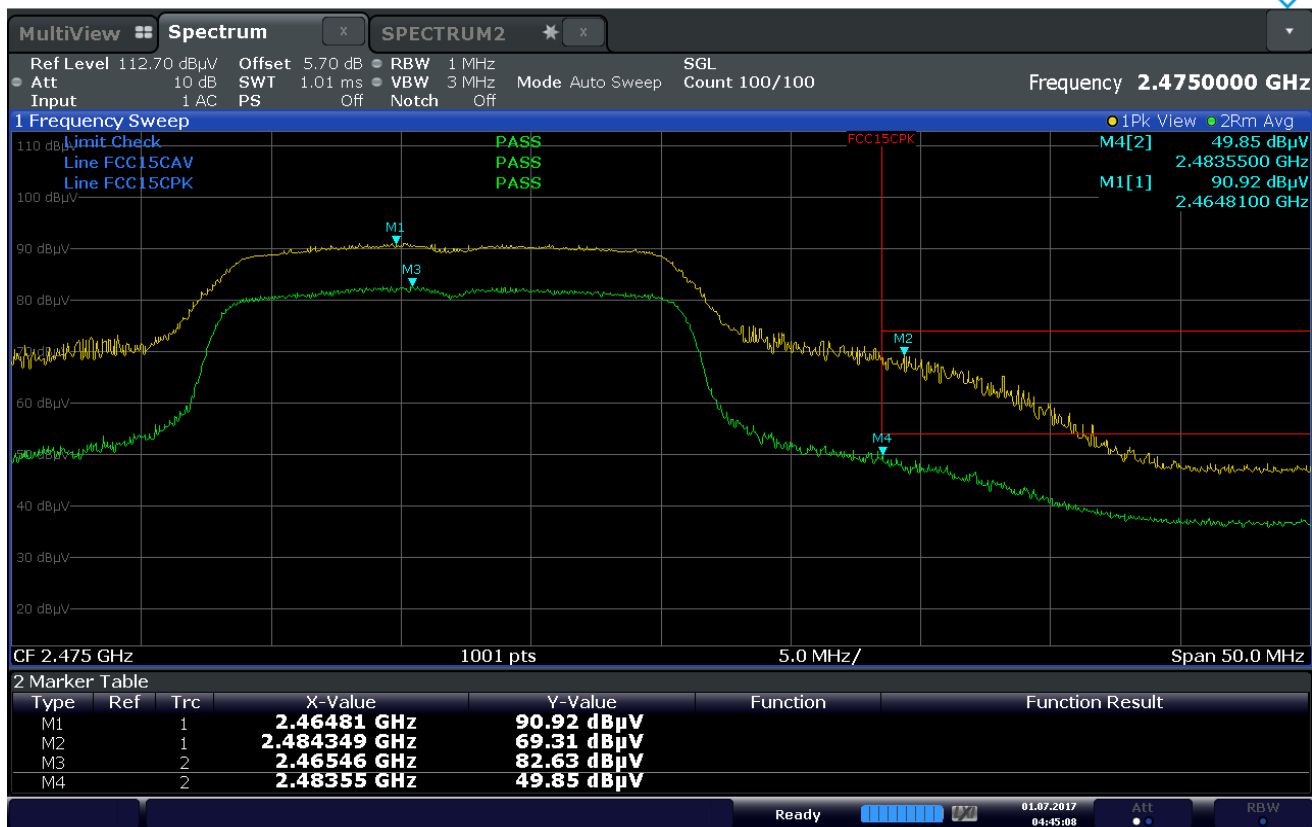
Plot 7-48. Radiated Restricted Upper Band Edge Measurement (Average & Peak)
