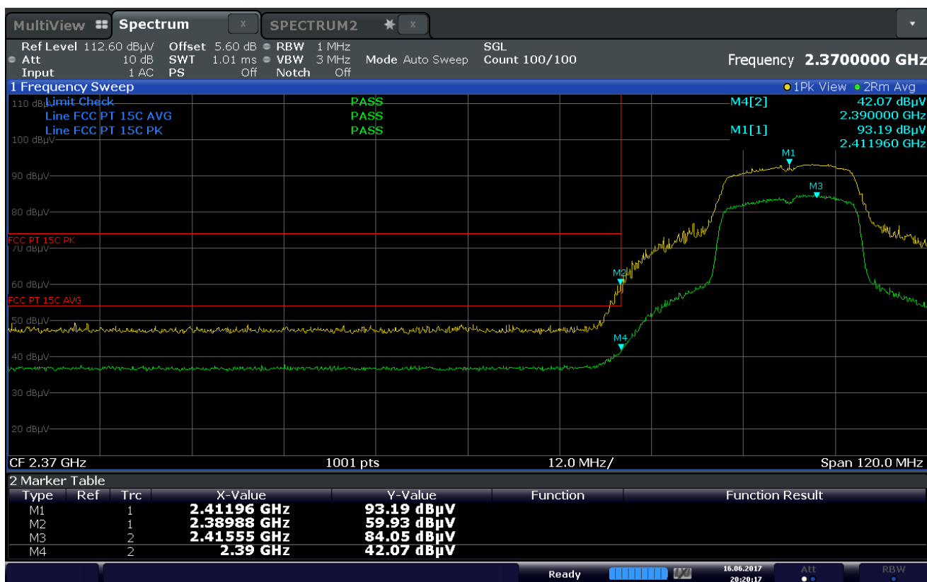
Plot 7-45. Radiated Restricted Lower Band Edge Measurement (Average & Peak)
