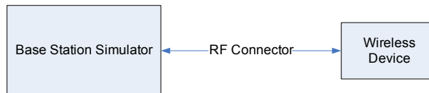
Figure 8-1 Power Measurement Setup
