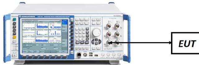
Figure 7-4. Conducted Power Measurement Setup
