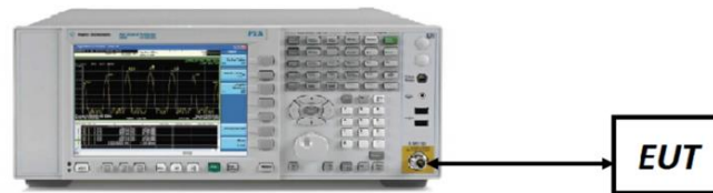
Figure 7-2. Test Instrument & Measurement Setup for Peak Power Measurement
