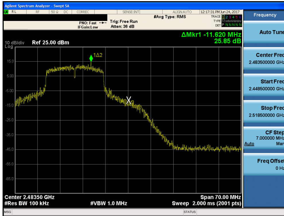
Plot 7-29. Band Edge Plot (802.11n (2.4GHz) – Ch. 12)
