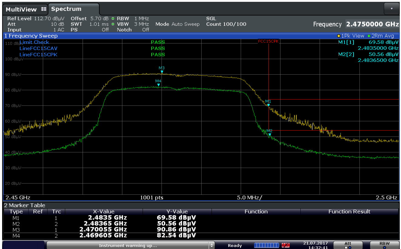
Plot 7-49. Radiated Restricted Upper Band Edge Measurement (Average & Peak)
