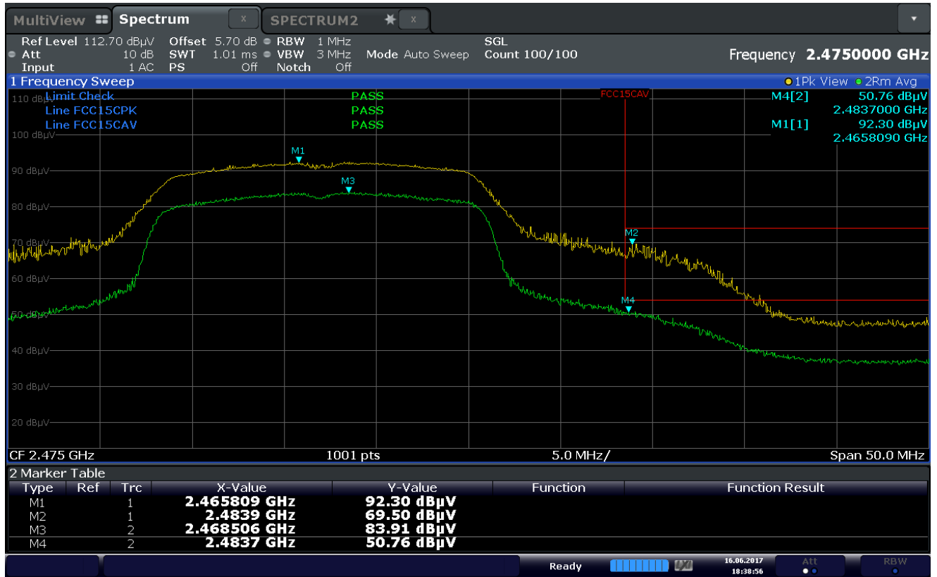
Plot 7-48. Radiated Restricted Upper Band Edge Measurement (Average & Peak)
