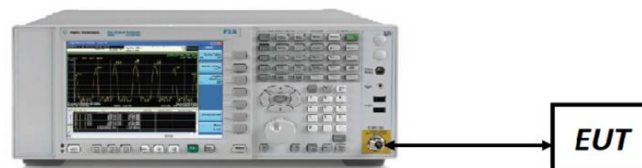
Figure 7-5. Test Instrument & Measurement Setup
