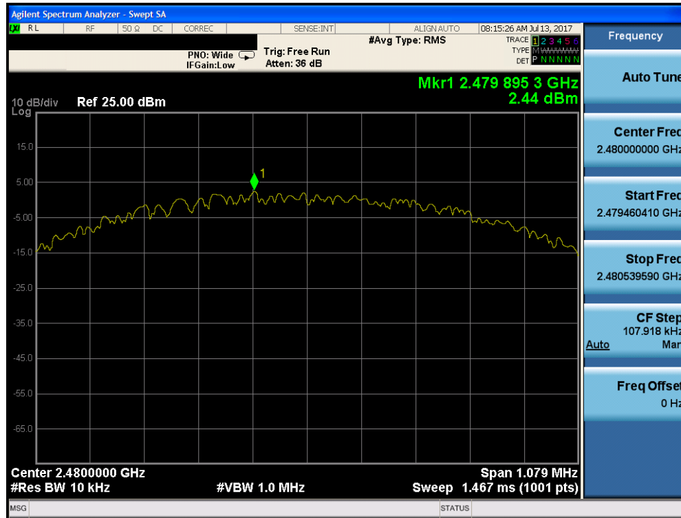
Plot 7-18. Power Spectral Density Plot (Bluetooth (LE), iPA – Ch. 39)
