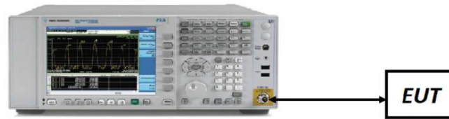
Figure 7-2. Test Instrument & Measurement Setup for Peak Power Measurement
