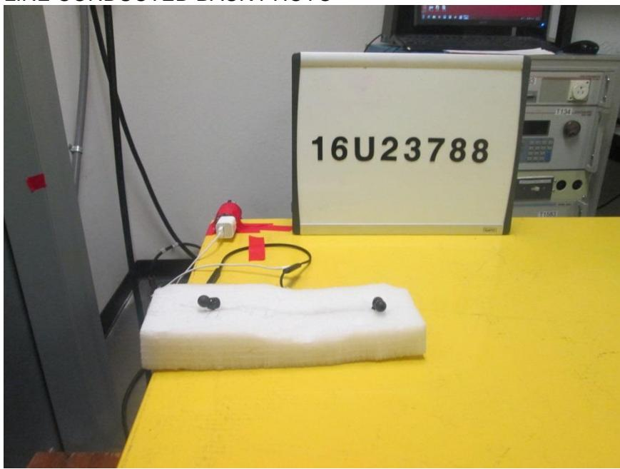
EUT POWERED BY HOST PC VIA USB CABLE
