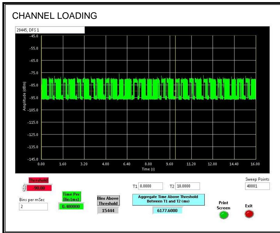
The level of traffic loading on the channel by the EUT is 61.77%
