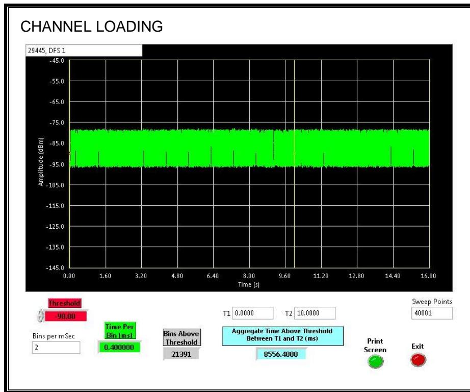
The level of traffic loading on the channel by the EUT is 85.56%
