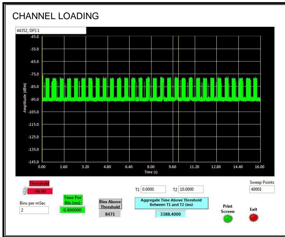
The level of traffic loading on the channel by the Peer Slave is 33.884%.
