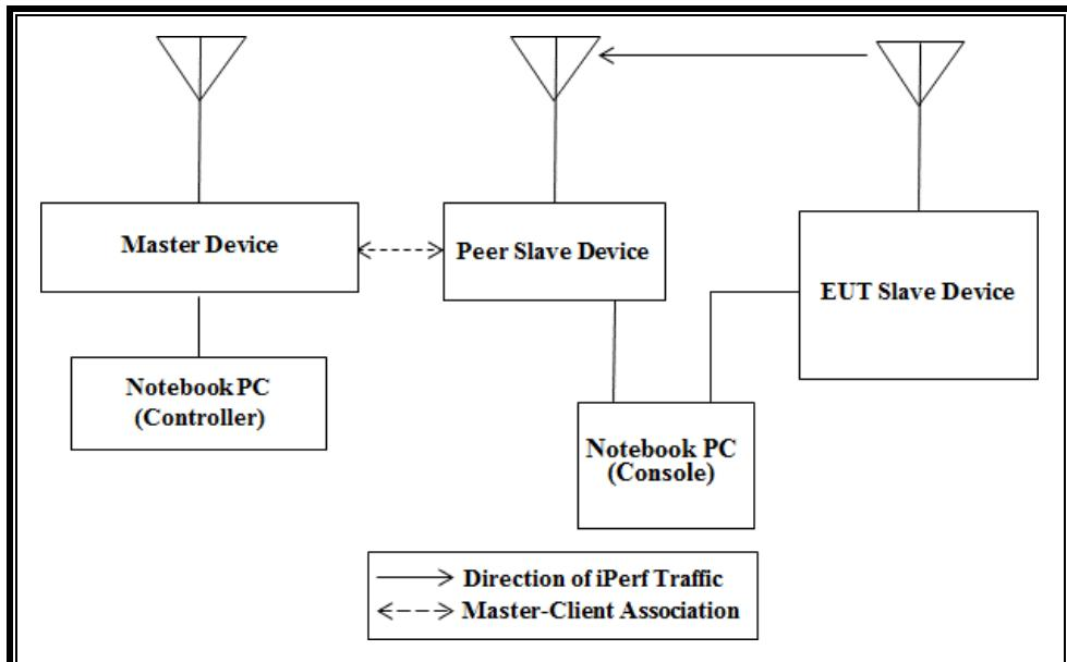
**RADIATED METHOD EUT TEST SETUP WHEN MONITORING THE PEER SLAVE DEVICE)**
