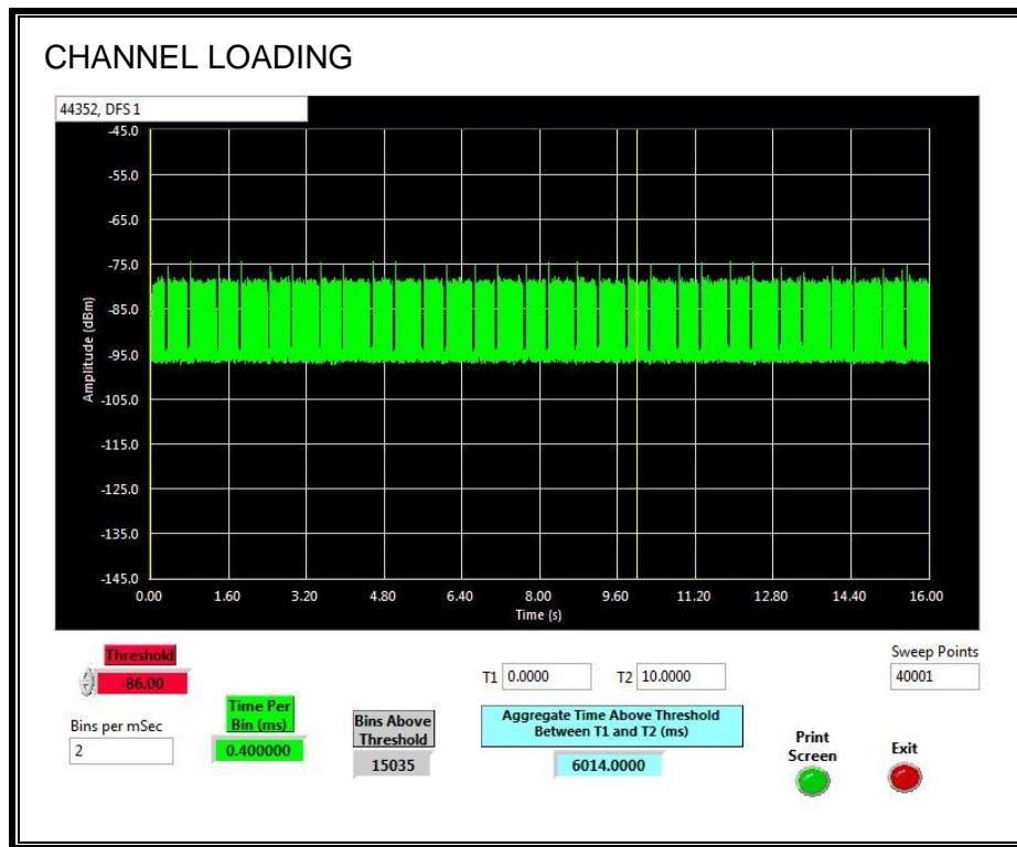
The level of traffic loading on the channel by the Peer Slave is 60.14%.
