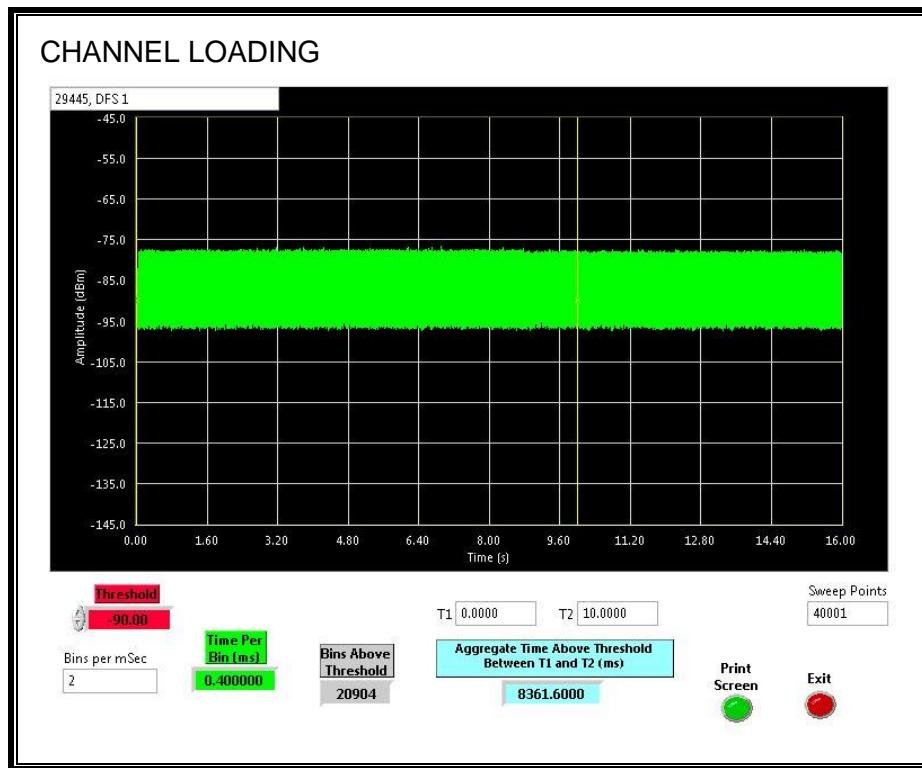
The level of traffic loading on the channel by the EUT is 83.61%
