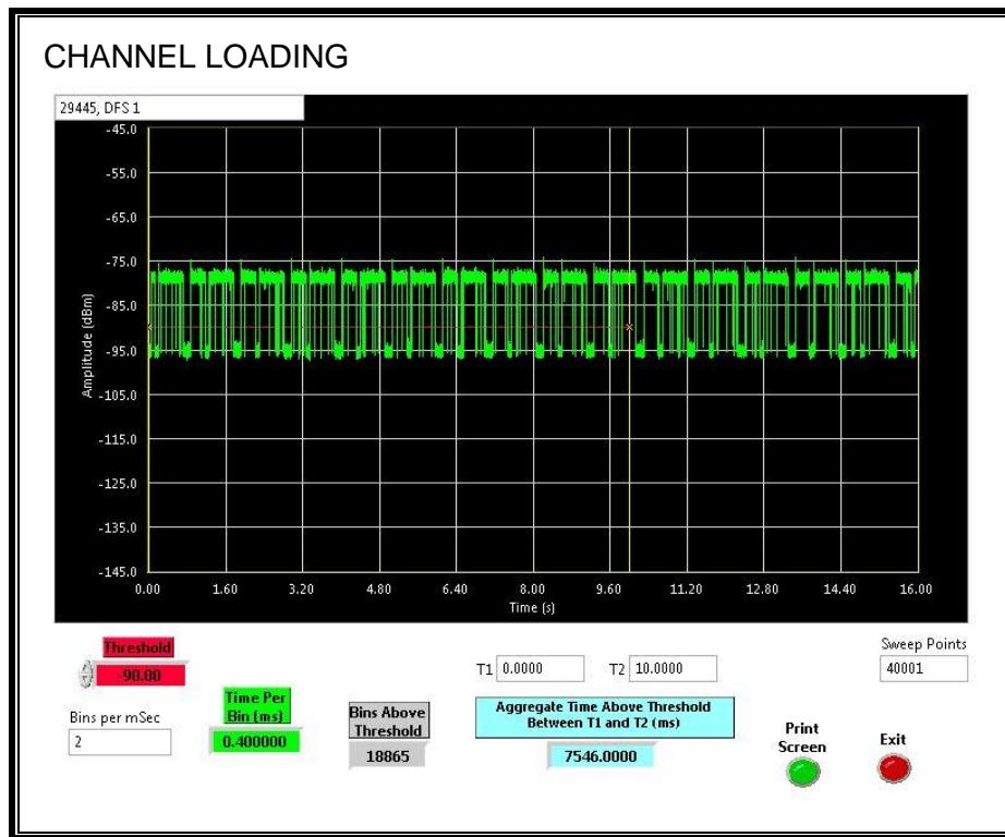
The level of traffic loading on the channel by the EUT is 75.46%
