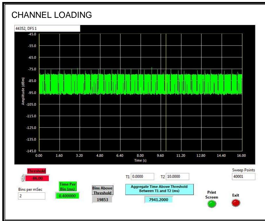
The level of traffic loading on the channel by the EUT is 79.412%.
