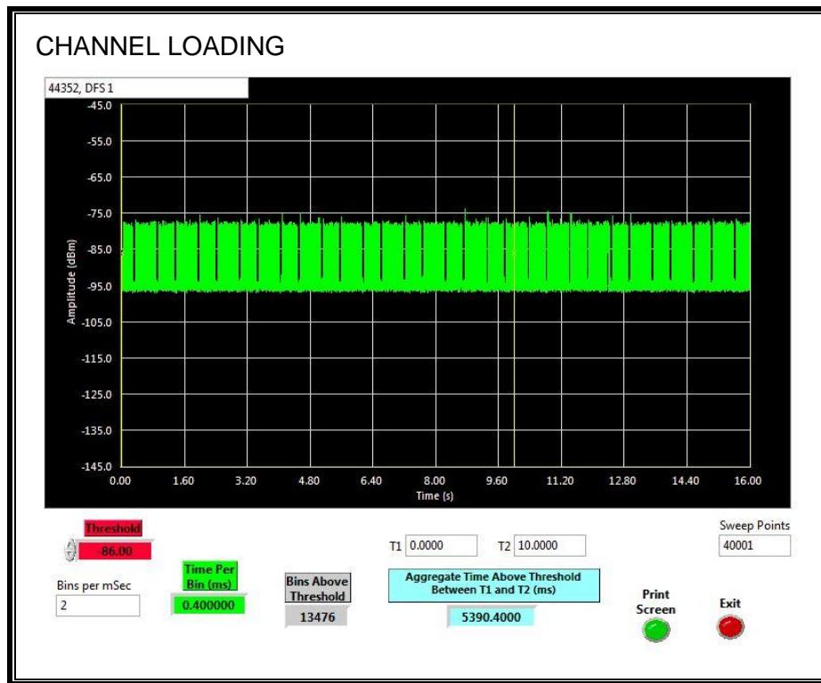
The level of traffic loading on the channel by the Peer Slave is 53.904%.
