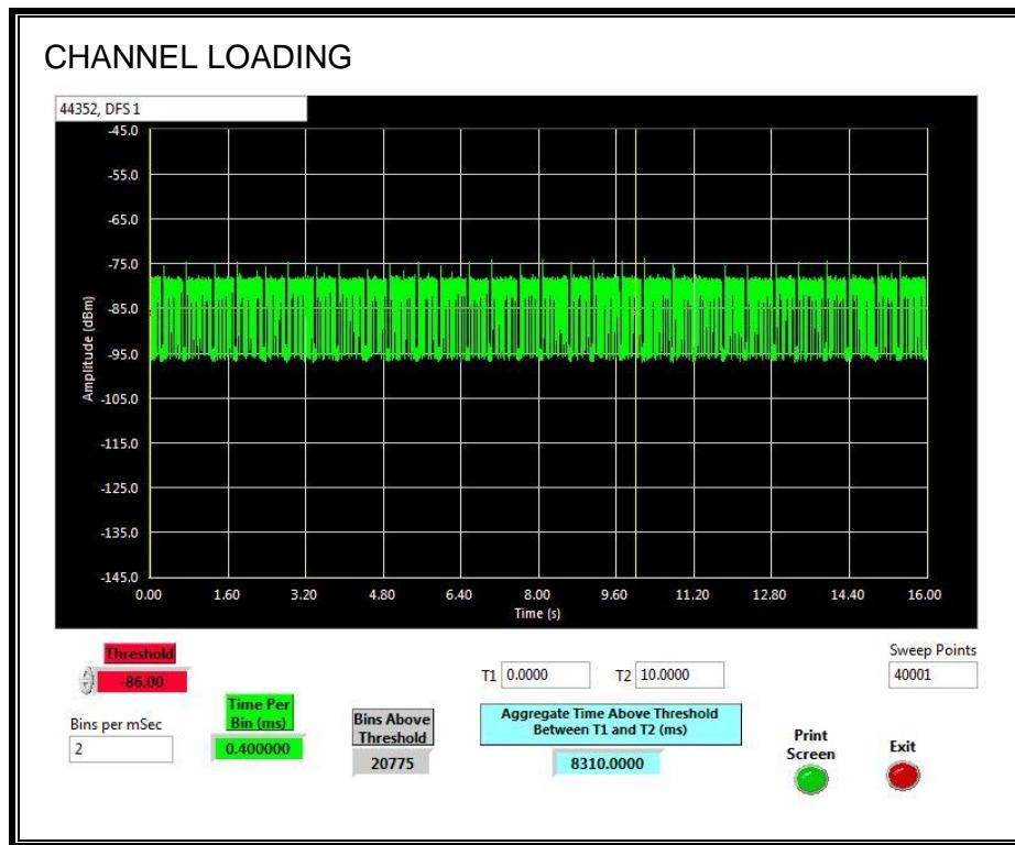
The level of traffic loading on the channel by the EUT is 83.1%.
