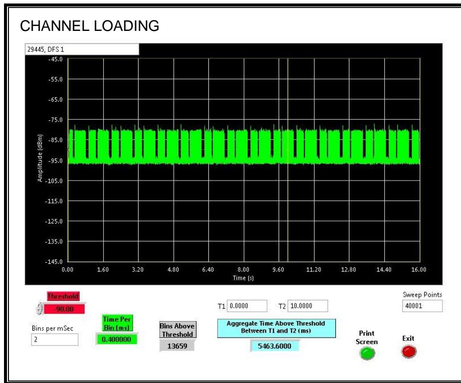
The level of traffic loading on the channel by the EUT is 54.63%
