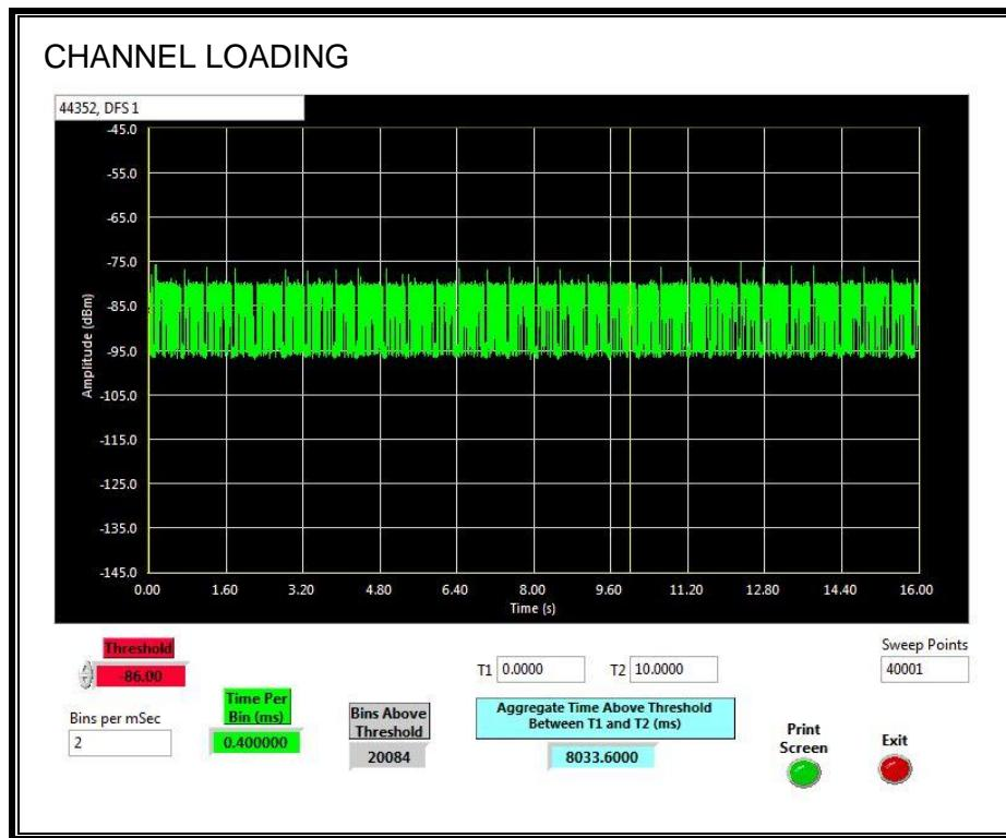
The level of traffic loading on the channel by the EUT is 80.336%
