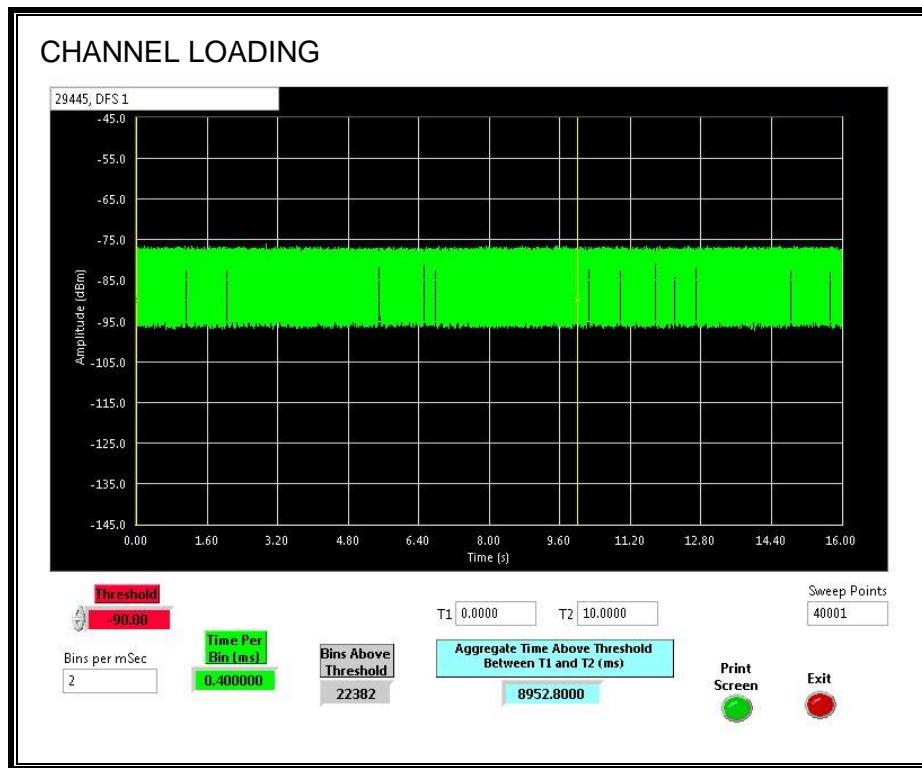
The level of traffic loading on the channel by the EUT is 89.52%
