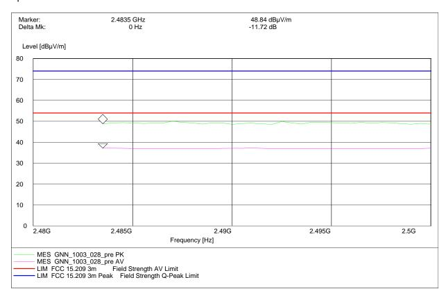
Radiated measurement (higher band edge)
