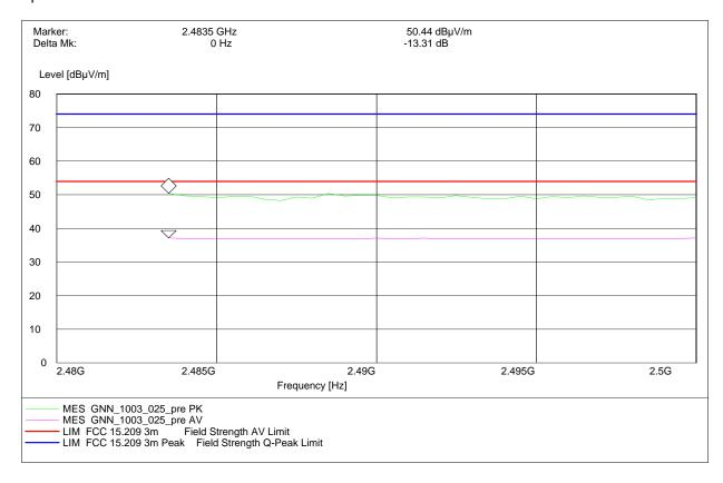
Radiated measurement (higher band edge)
