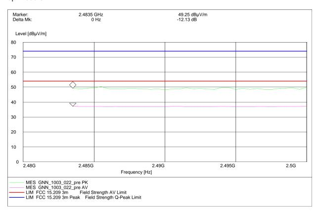
Radiated measurement (higher band edge)
