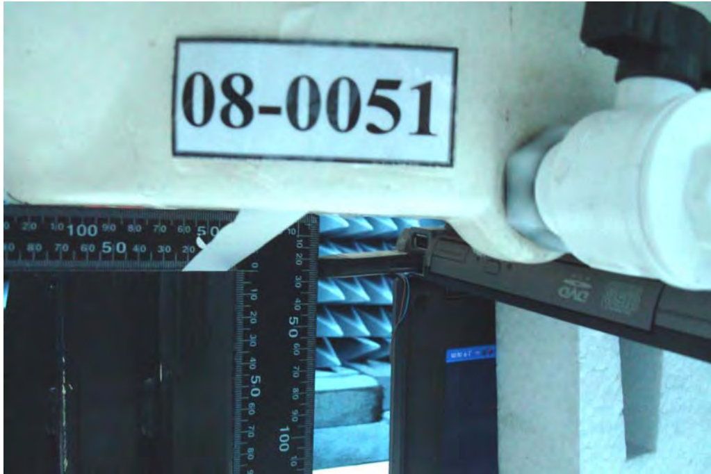
Figure 13. Body SAR Test Setup _ EUT Bottom to phantom close Body ( NB3 )
