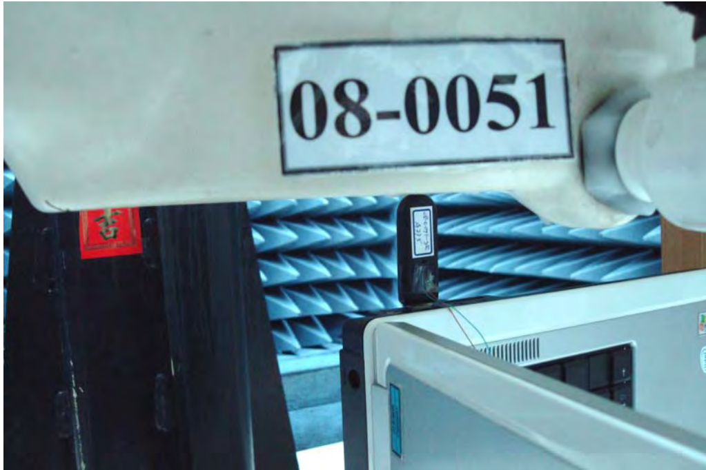
Figure 15. Body SAR Test Setup _ EUT Tip to phantom close Body ( NB2 )
