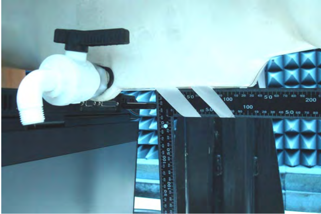
Figure 11.Body SAR Test Setup _ EUT Bottom to phantom close Body ( NB1 )
