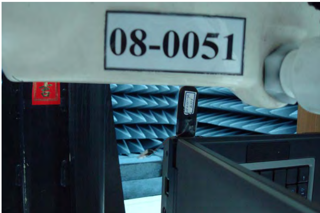
Figure 16. Body SAR Test Setup _ EUT Tip to phantom close Body ( NB3 )
