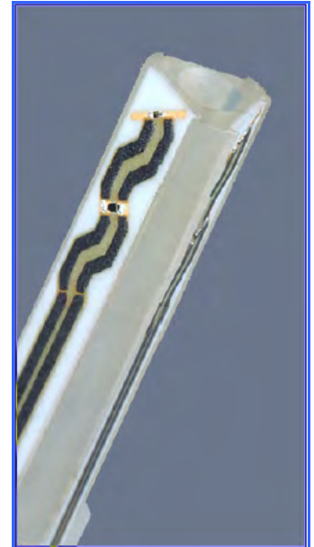
Figure 4. EX3DV3 E-field Probe
