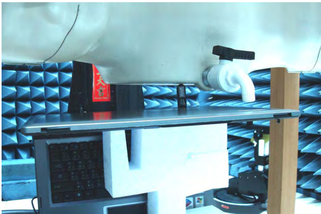
Figure 14. Body SAR Test Setup _ EUT Tip to phantom close Body ( NB1 )
