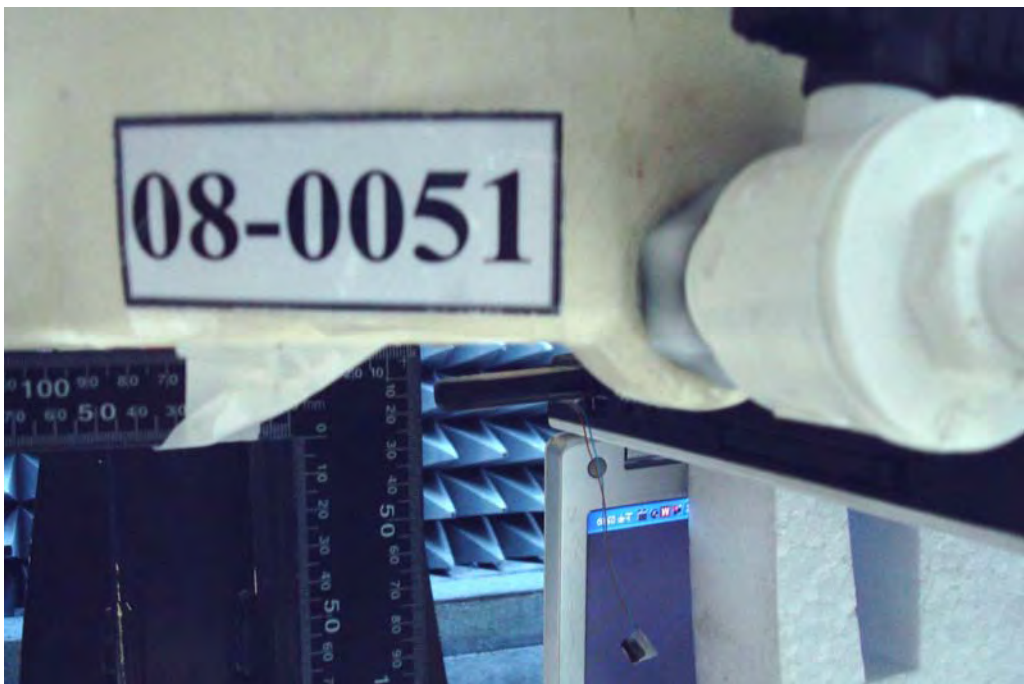
Figure 12.Body SAR Test Setup _ EUT Bottom to phantom close Body ( NB2 )
