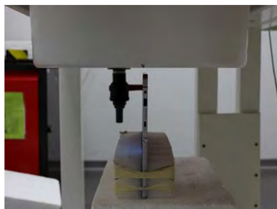
Fig.7 EUT Top side (10mm) to flat phantom
