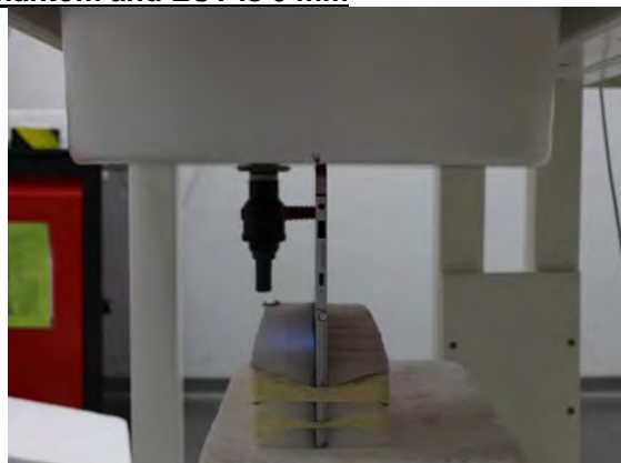
Fig.6 EUT Top side to flat phantom
