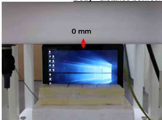
Fig.6 EUT Top side to flat phantom
