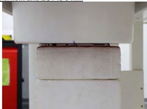
Fig.3 EUT Back side to flat phantom
