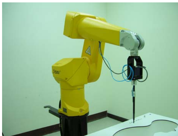
Fig. 5.2 Probe setup on robot
