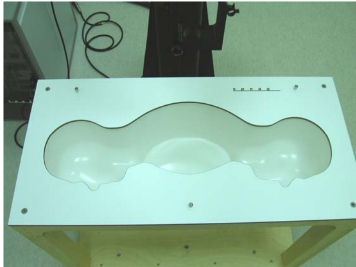
Fig. 5.3 Top view of twin phantom
