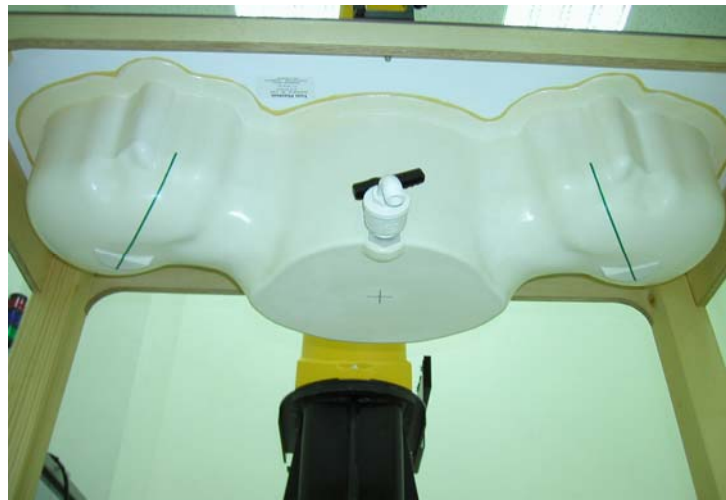
Fig. 5.4 Bottom view of twin phantom
