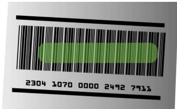
The green light bar should be approximately centered on the bar code and cover approximately 3/4 of a wide bar code
