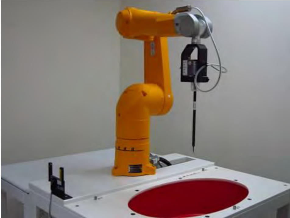
Fig.1 Photograph of the SAR measurement system
