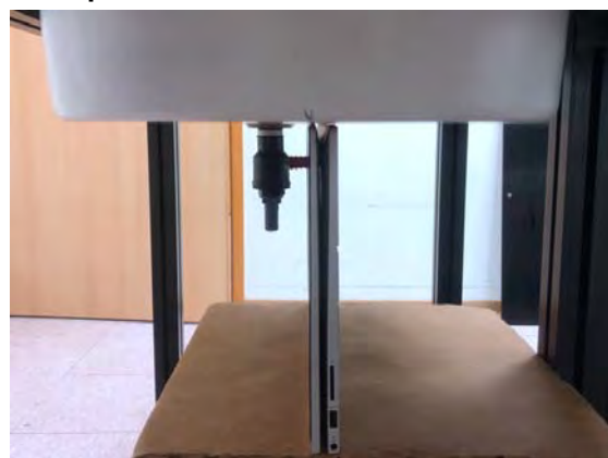
Fig.4 EUT Top side to flat phantom
