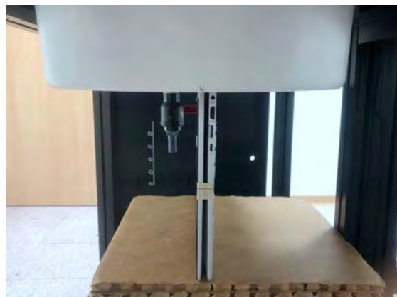
Fig.5 EUT Bottom side to flat phantom
