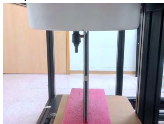
Fig.7 EUT Left side to flat phantom
