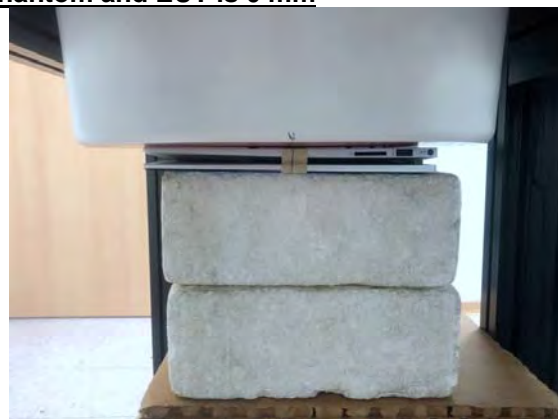
Fig.3 EUT Back side to flat phantom
