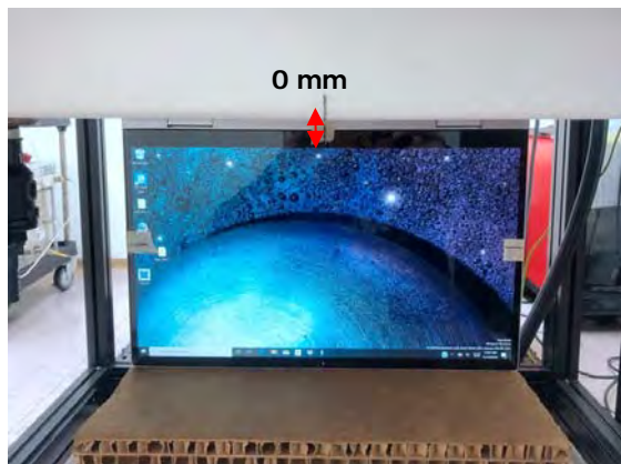
Fig.5 EUT Bottom side to flat phantom
