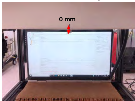
Fig.4 EUT Top side to flat phantom
