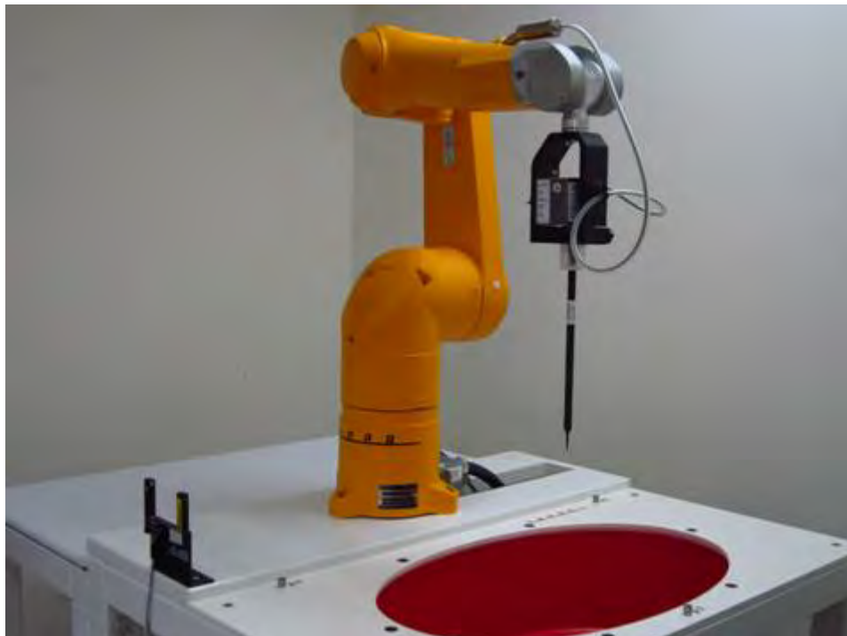
Fig.1 Photograph of the SAR measurement system
