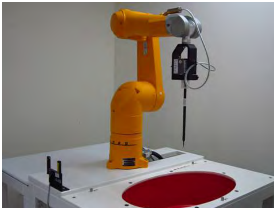
Fig.1 Photograph of the SAR measurement system
