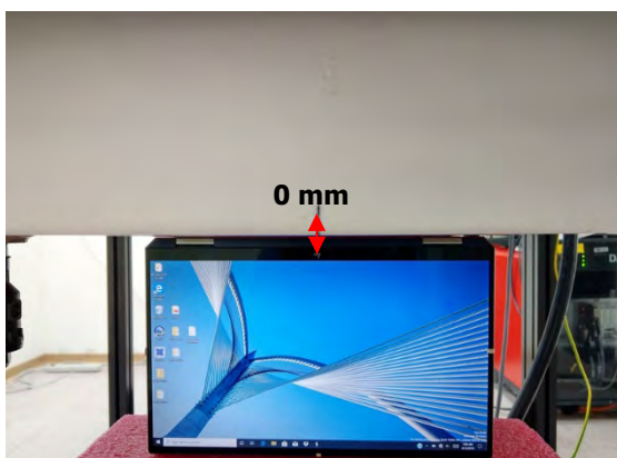
Fig.5 EUT Bottom side to flat phantom
