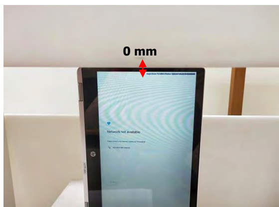
Fig.7 EUT Left side to flat phantom
