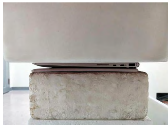
Fig.3 EUT Back side to flat phantom
