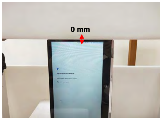
Fig.6 EUT Right side to flat phantom
