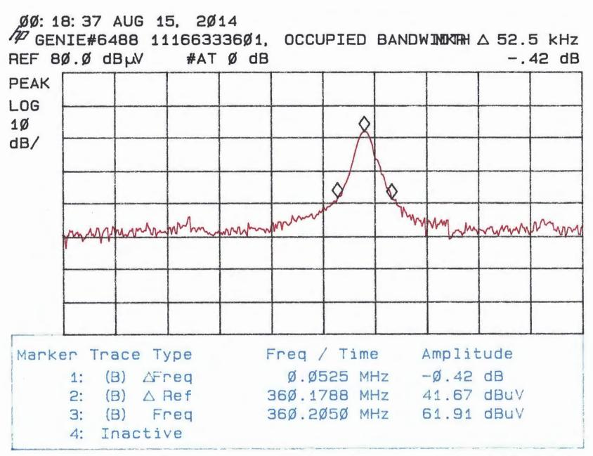
CENTER 36Ø.165Ø MHz #RES BW 10 kHz VBW 10 kHz SWP 30.0 msec
