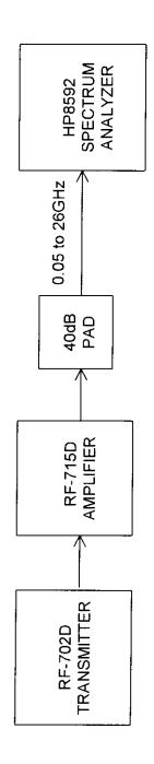
FIGURE 1 - SPURIOUS EMISSION AT ANTENNA TEST SET-UP
