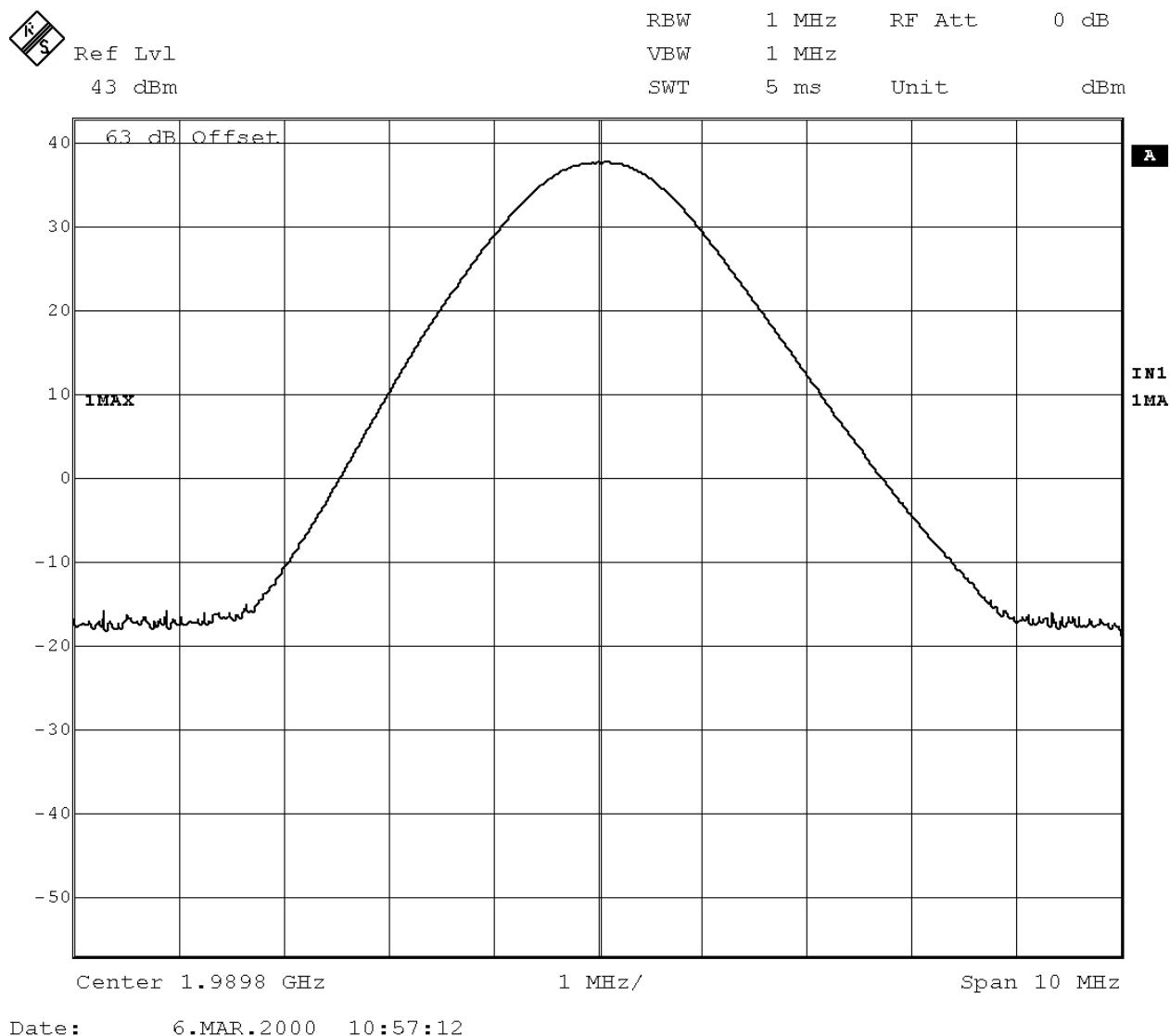
Channel 810 / Carrier frequency = 1989.8 MHz
