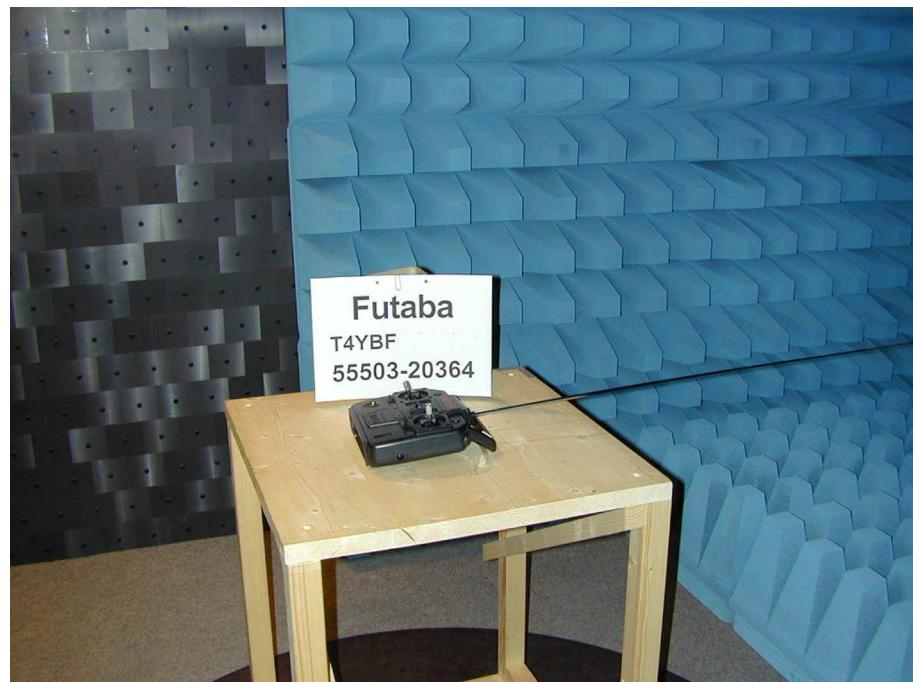
**Test setup for radiated emission measurement
