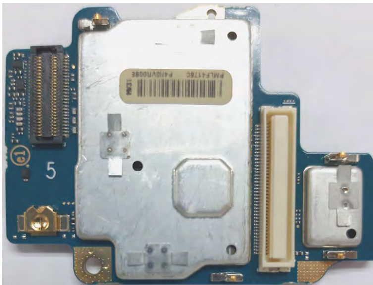
Vocon board with shields (Bottom) (APX6000/APX5000/APX6000XE/APX6000Li/SRX2200)
