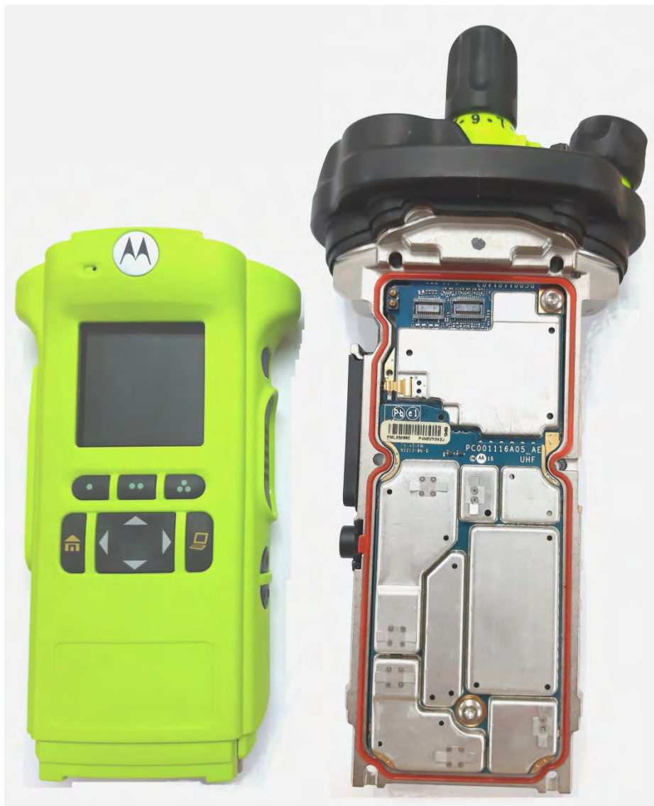
RF and Vocon boards with chassis and housing of APX6000XE Model 2.5 (Front side)
