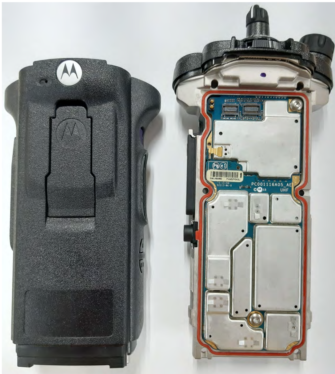
RF and Vocon boards with chassis and housing of APX6000/APX6000Li/APX5000 Model 1.5 (Front side)
