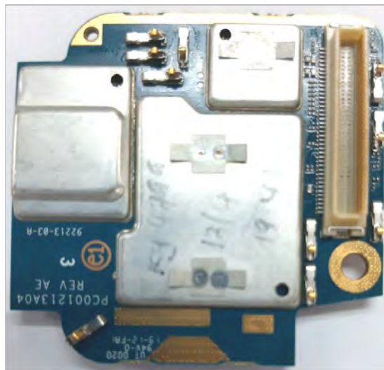
Expansion board with shields (Bottom) (APX6000/APX5000/APX6000XE/APX6000Li/SRX2200)
