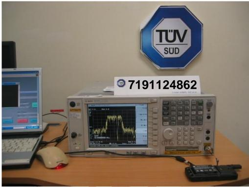
**Peak Power Spectral Density Test Setup**
