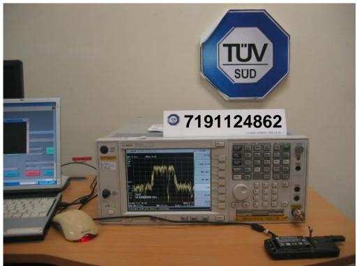
**Carrier Frequency Separation Test Setup**
