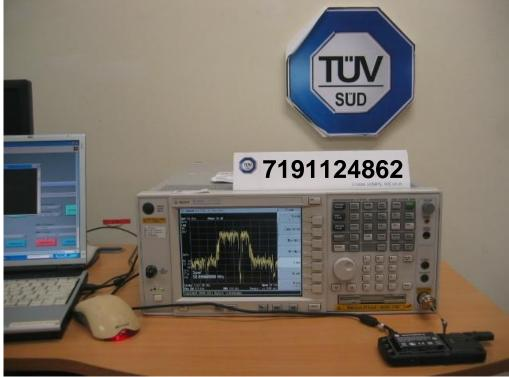
Spectrum Bandwidth (20dB Bandwidth Measurement) Test Setup
