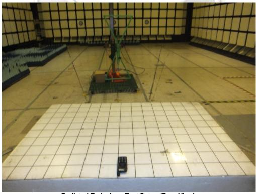
Radiated Emissions Test Setup (Rear View)
