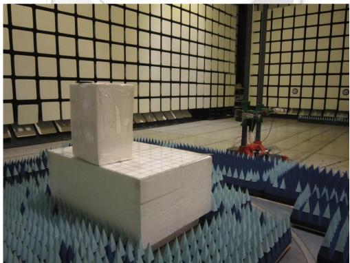
Radiated Emissions Test Setup (Rear View)
