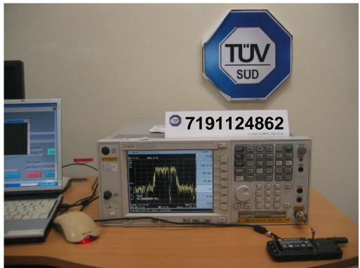
Band Edge Compliance (Conducted) Test Setup
