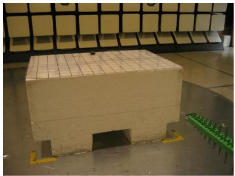
Radiated Emissions Test Setup (Front View)
