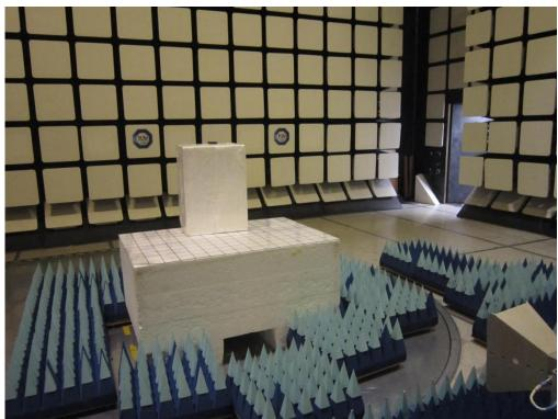
Radiated Emissions Test Setup (Front View)
