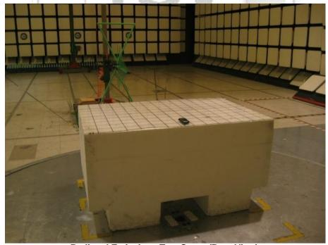
Radiated Emissions Test Setup (Rear View)
