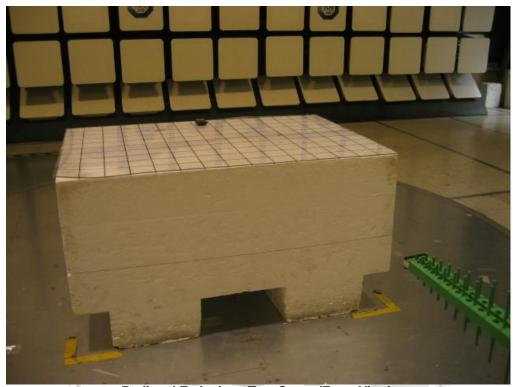
Radiated Emissions Test Setup (Front View)
