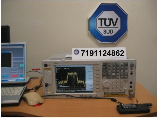
**RF Conducted Spurious Emissions Test Setup**
