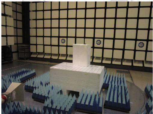
Band Edge Compliance (Radiated) Test Setup
