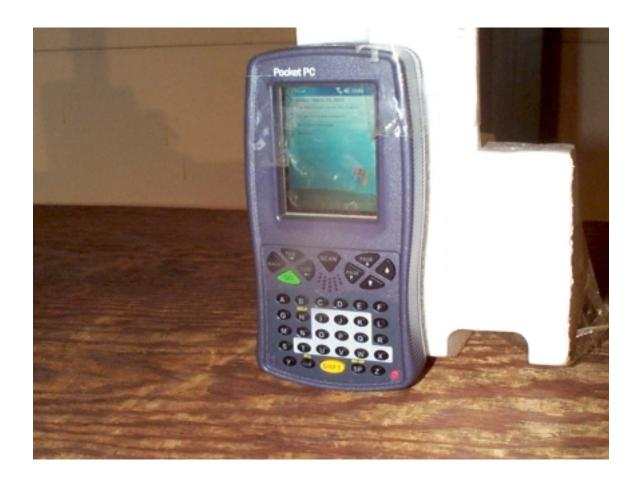
Photo 2 of 3 -Front View of PowerPad With Foam Support To Hold The Terminal Upright While measuring emissions under Part 22 & 24
