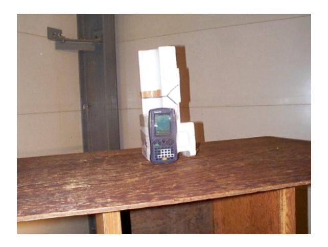
Photo 3 of 3 - View of Enhanced PowerPad Terminal On It's Back as it was when measureing the Bluetooth emissions under Part 15.
