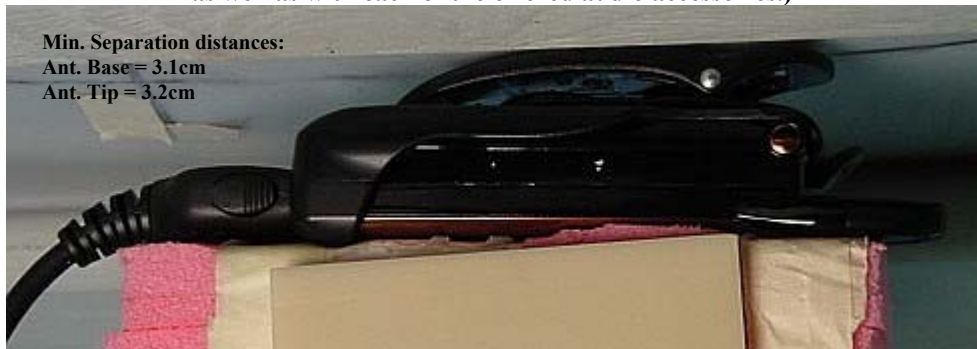
Figure 7. Assessment @ Body; antenna retracted. DUT with belt clip model NNTN5002A against the flat phantom and attached data cable model NKN6560A. (Same position used with antenna extended, with and without a data cable attached, as well as with each of the offered audio accessories.)
