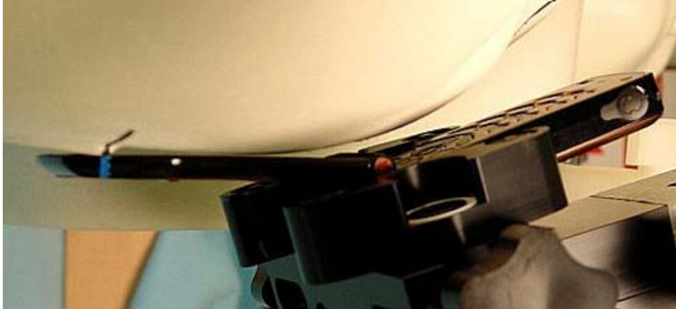
Figure 5. Assessment @ the Right ear; antenna retracted. DUT in cheek touch position. (Same position used for antenna extended.)
