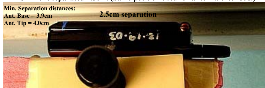
Figure 9. Assessment @ the Body; antenna retracted. DUT front separated 2.5cm. (Same position used for antenna extended.)
