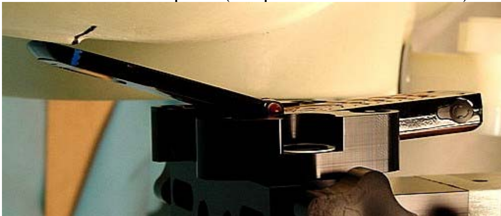
Figure 4. Assessment @ the Right ear; antenna retracted. DUT in 15° tilt position. (Same position used for antenna extended.)
