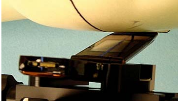
Figure 2. Assessment @ the Left ear; antenna retracted. DUT in 15° tilt position. (Same position used for antenna extended.)
