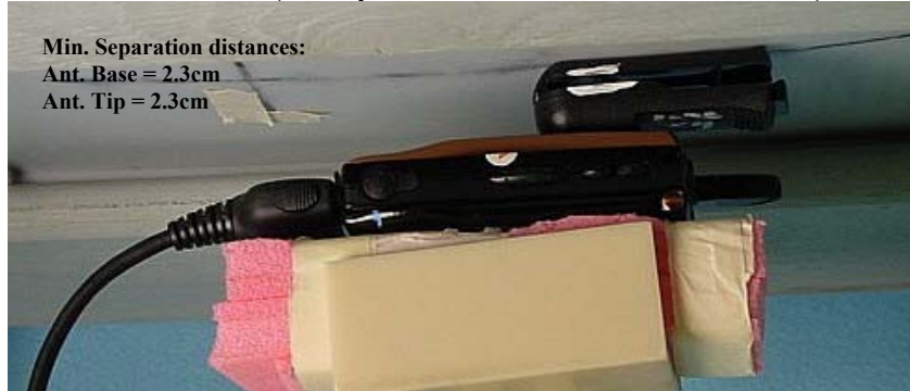
Figure 9. Assessment @ the Body; antenna retracted. DUT front separated 2.5cm. (Same position used for antenna extended.)
