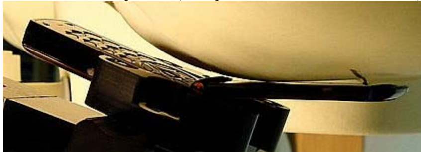
Figure 3. Assessment @ the Left ear; antenna retracted. DUT in cheek touch position. (Same position used for antenna extended.)
