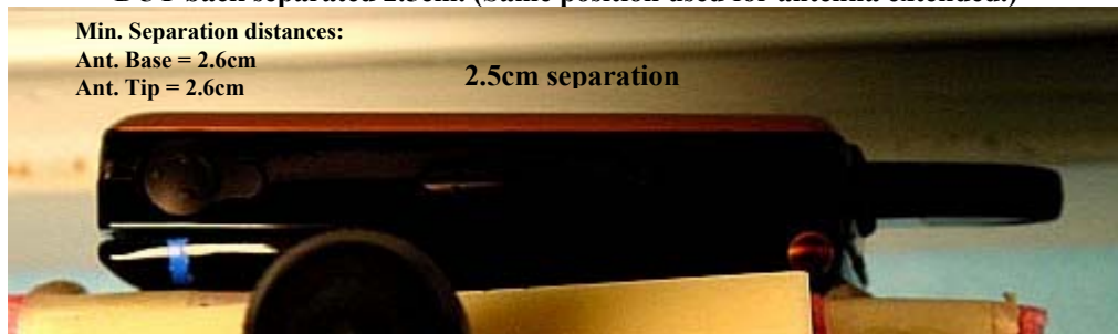
Figure 10. Assessment @ the Body; antenna retracted. DUT back separated 2.5cm. (Same position used for antenna extended.)
