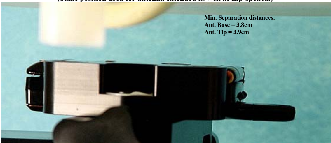
Figure 6. Assessment @ the Face; antenna retracted. DUT front 2.5cm separation distance from flat area of the SAM phantom with the flip closed. (Same position used for antenna extended as well as flip opened.)
