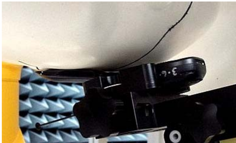
Figure 7. Assessment @ the Right ear; Cheek touch position with antenna extended. Same position used for antenna retracted.
