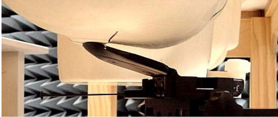
Figure 8. Assessment @ the Right ear; 15 degrees tilt position with antenna extended. Same position used for antenna retracted.
