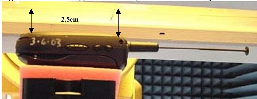
Figure 9. Assessment @ the Abdomen; DUT back 2.5cm separation distance
