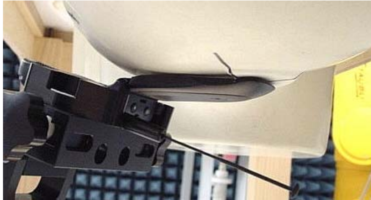
Figure 5. Assessment @ the Left ear; Cheek touch position with antenna extended. Same position used for antenna retracted.
