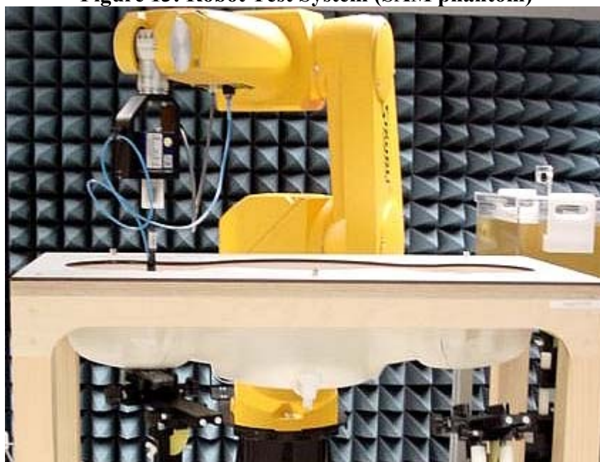
Figure 13: Robot Test System (SAM phantom)
