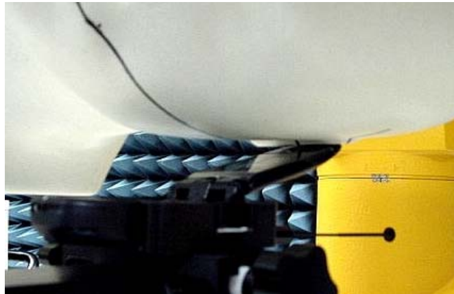
Figure 6. Assessment @ the Left ear; 15 degrees tilt position with antenna extended. Same position used for antenna retracted.
