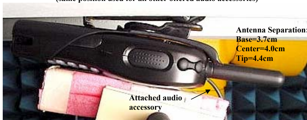
Figure 4. Assessment at the body; Belt clip against the phantom with attached HMN9039B audio accessory (same position used for all other offered audio accessories)
