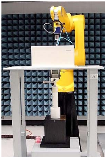
Figure 10: Robot Test Setup 2.4GHz band (Body)
