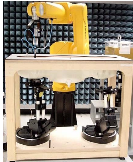
Figure 11: Robot Test Setup 2.4GHz band (Head)
