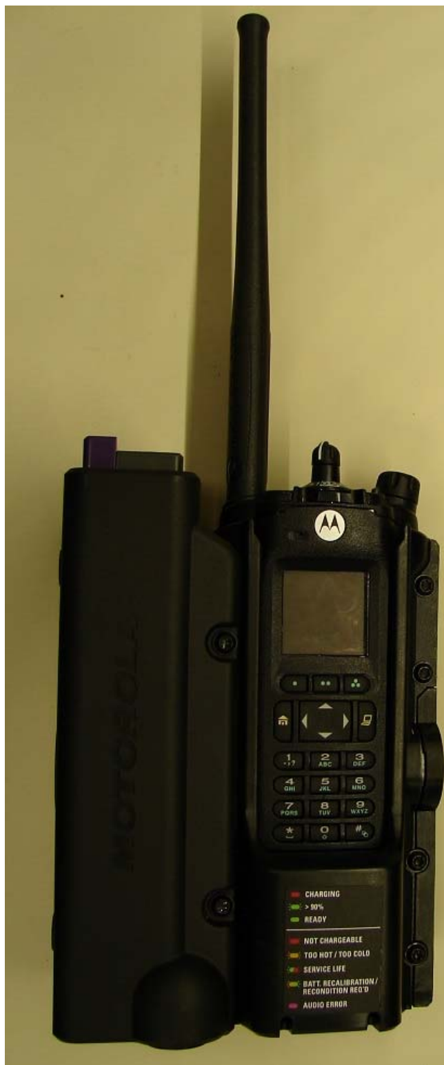
NNTN8527A with radio installed
