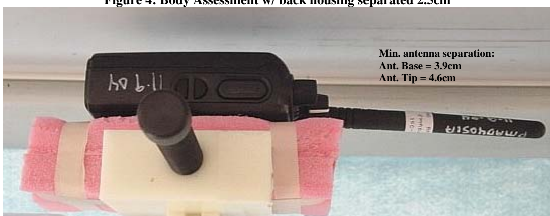
Figure 5: Body Assessment w/ antenna (back towards phantom) separated 2.5cm
