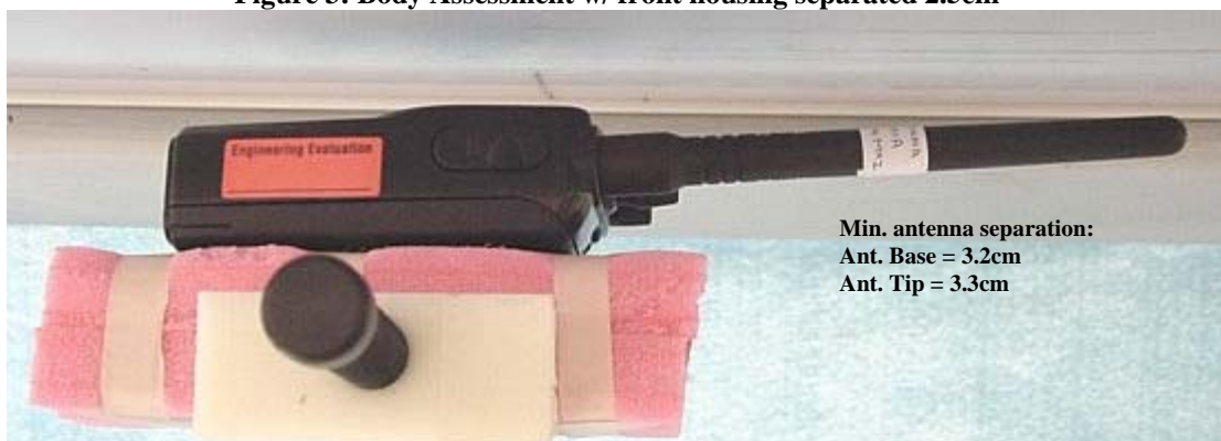
Figure 4: Body Assessment w/ back housing separated 2.5cm
