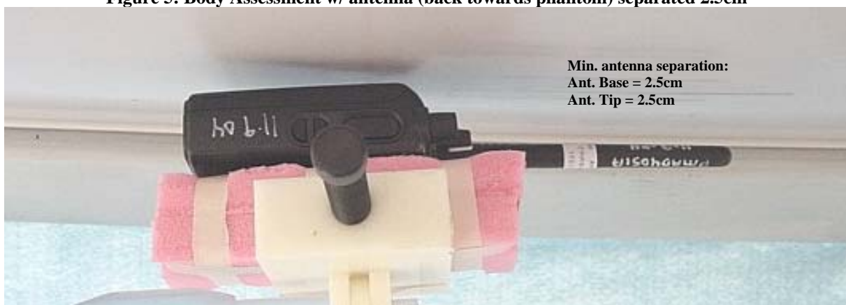
Figure 5: Body Assessment w/ antenna (back towards phantom) separated 2.5cm
