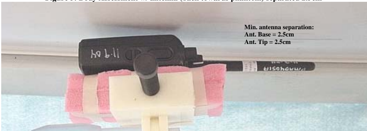
Figure 5: Body Assessment w/ antenna (back towards phantom) separated 2.5cm
