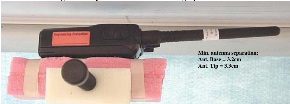
Figure 4: Body Assessment w/ back housing separated 2.5cm
