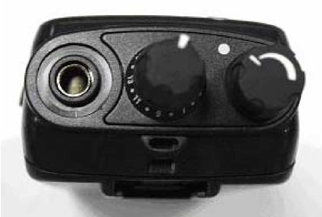
Figure 3-6: Top view of complete radio.
