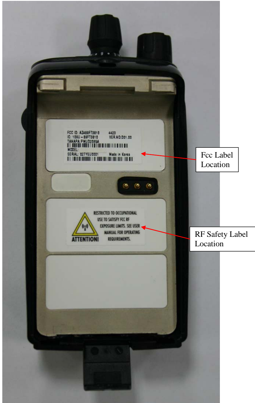
Figure 3-5: Rear view of complete radio showing FCC Label & RF Safety Label location.
