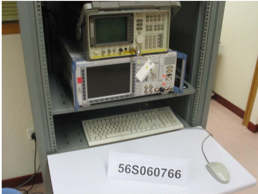
Carrier Frequency Separation Test Setup
