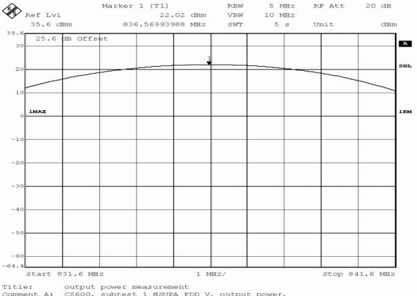
Comment A: CZ600, subtest 1 HSUPA FDD V, output power, channel 4183 (836.6MHz)
