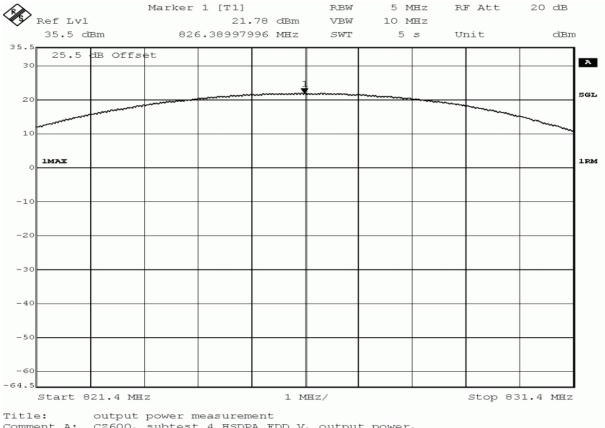
Comment A: CZ600, subtest 4 HSDPA FDD V, output power, channel channel 4132 (826.4MHz)
