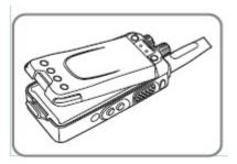
Push the battery pack to the connection of chassis and push down the battery locker
