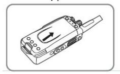
To remove the battery pack, pull up the battery locker and slide the pack away from the transceiver.
