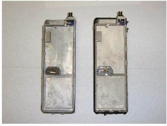
The following two photographs show the chassis with installed PC boards. As can be seen the internal design is unaltered. There is a difference in the shield cover arrangement. The new design features a single piece shield with improved grounding to the chassis. The result is a mechanical construction offering equal performance to the original design.
