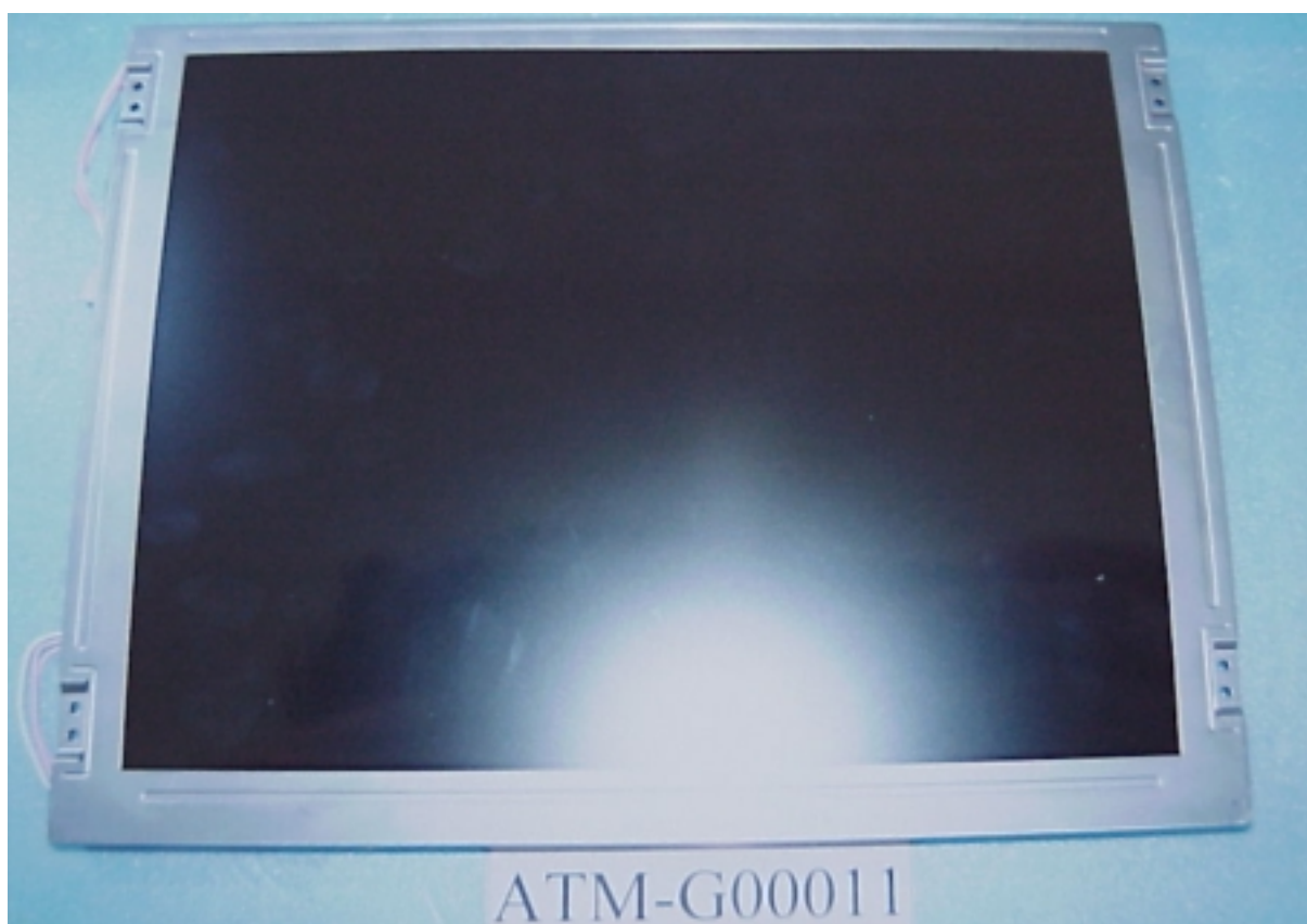
Figure 6 Hyundai LCD Panel (Front View)
