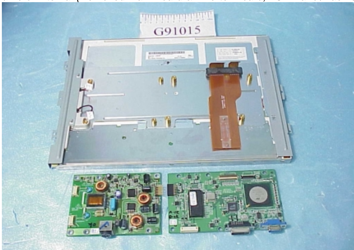
Figure 28 Frame of Internal (Removed Main Board & Inverter Board, LCD Panel/Back Side)
