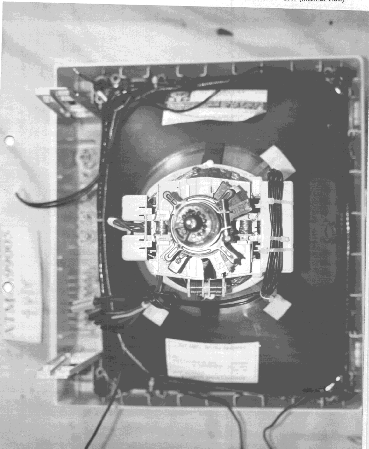
Figure 3 Frame of 14" CRT (Internal View)
