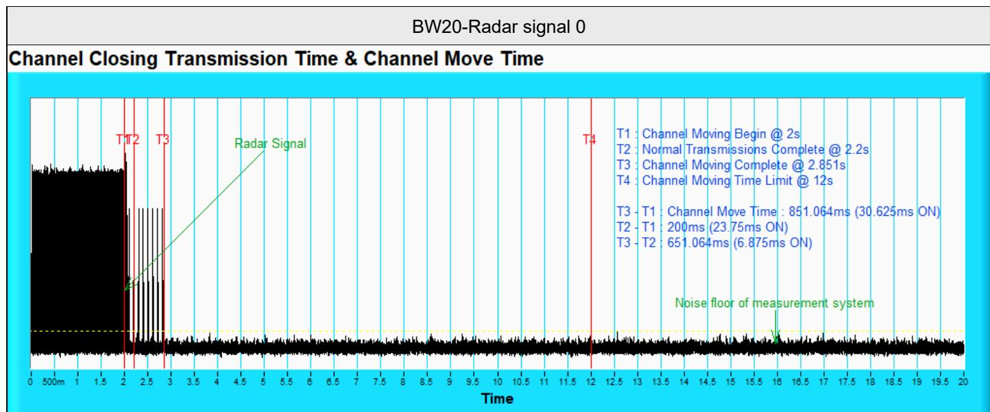
Note: T1 denotes the start of Channel Move Time upon the end of the last Radar burst. T2 denotes the data transmission time of 200 ms from T1. T3 denotes the end of Channel Move Time. T4 denotes the 10 second from T1 to observe the aggregate duration of transmissions.
