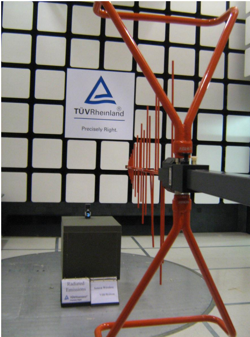
Figure 2: Test Setup for 30 MHz to 1000MHz (Rear View)
